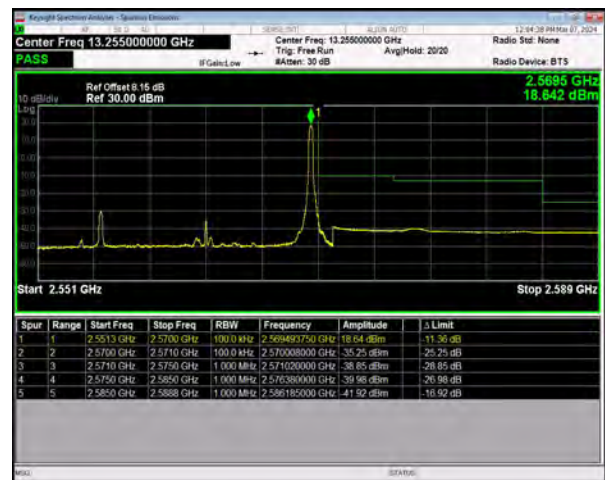
n7 SCS=15kHz DFT_16QAM BW=15MHz HighChannel=512500 RB=1@78
