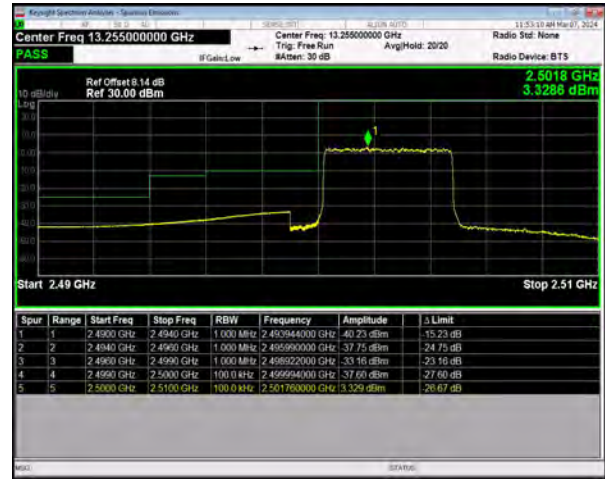
n7 SCS=15kHz DFT_64QAM BW=5MHz LowChannel=500500 RB=25@0
