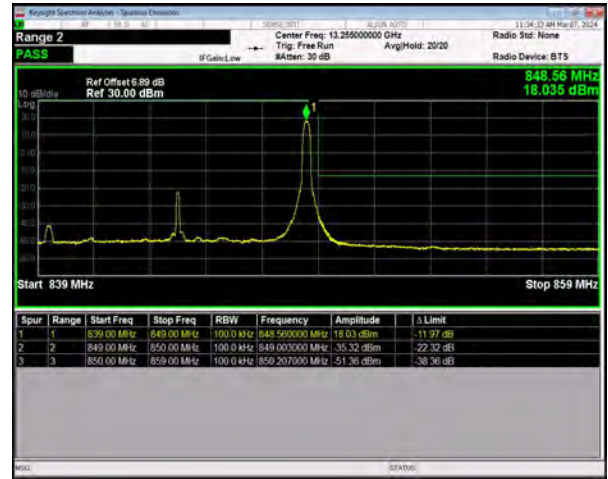
n5 SCS=15kHz DFT_16QAM BW=10MHz HighChannel=168800 RB=1@51
