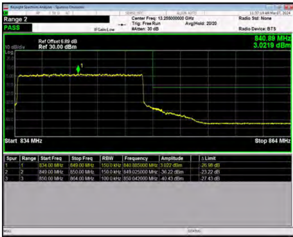
n5 SCS=15kHz DFT_BPSK BW=15MHz HighChannel=168300 RB=75@0
