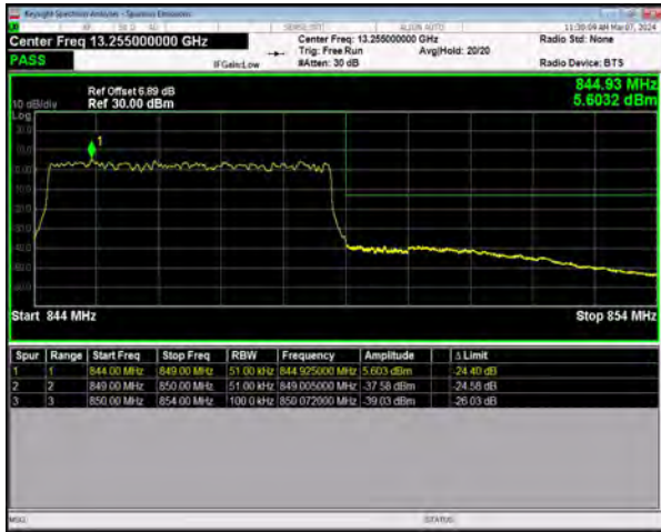
n5 SCS=15kHz DFT_64QAM BW=5MHz HighChannel=169300 RB=25@0
