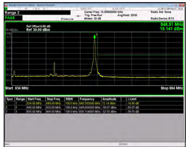
n5 SCS=15kHz DFT_256QAM BW=15MHz HighChannel=168300 RB=1@78
