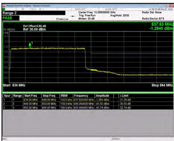
n5 SCS=15kHz DFT_256QAM BW=15MHz HighChannel=168300 RB=75@0
