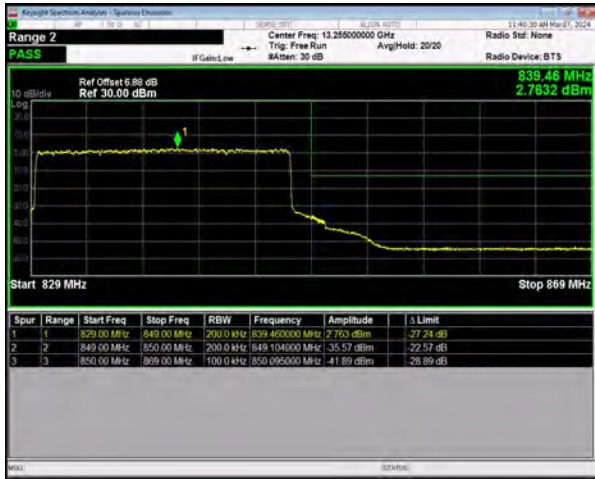
n5 SCS=15kHz DFT_BPSK BW=20MHz HighChannel=167800 RB=100@0
