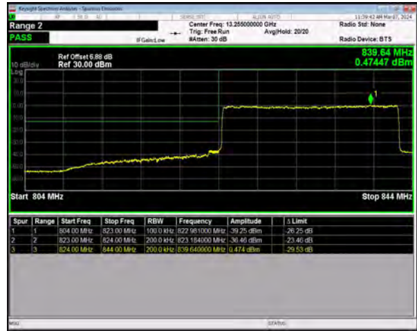
n5 SCS=15kHz DFT_64QAM BW=20MHz LowChannel=166800 RB=100@0
