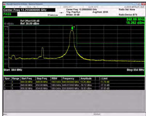
n5 SCS=15kHz DFT_16QAM BW=5MHz HighChannel=169300 RB=1@24
