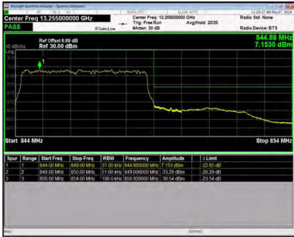
n5 SCS=15kHz DFT_BPSK BW=5MHz HighChannel=169300 RB=25@0
