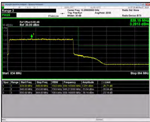
n5 SCS=15kHz DFT_QPSK BW=15MHz HighChannel=168300 RB=75@0
