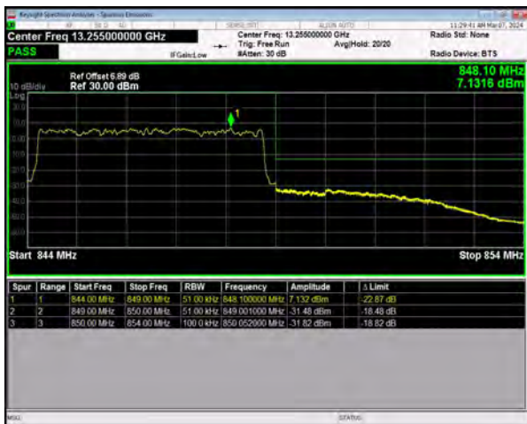
n5 SCS=15kHz DFT_QPSK BW=5MHz HighChannel=169300 RB=25@0
