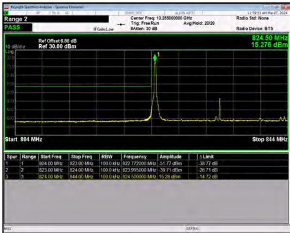
n5 SCS=15kHz DFT_256QAM BW=20MHz LowChannel=166800 RB=1@0
