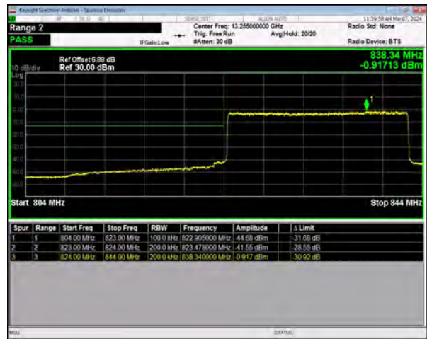
n5 SCS=15kHz DFT_256QAM BW=20MHz LowChannel=166800 RB=100@0
