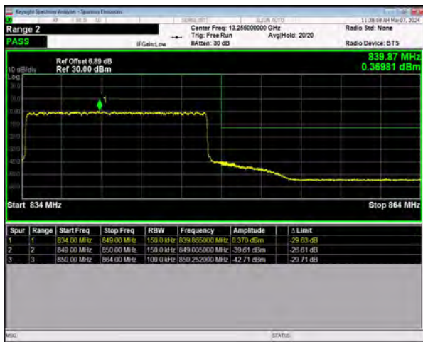
n5 SCS=15kHz DFT_64QAM BW=15MHz HighChannel=168300 RB=75@0
