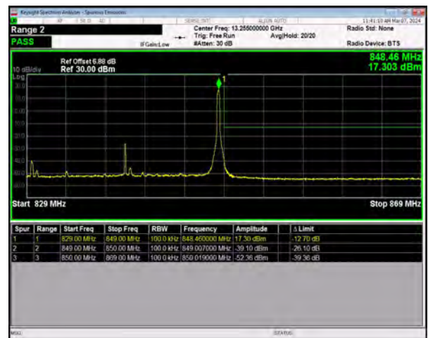
n5 SCS=15kHz DFT_64QAM BW=20MHz HighChannel=167800 RB=1@105
