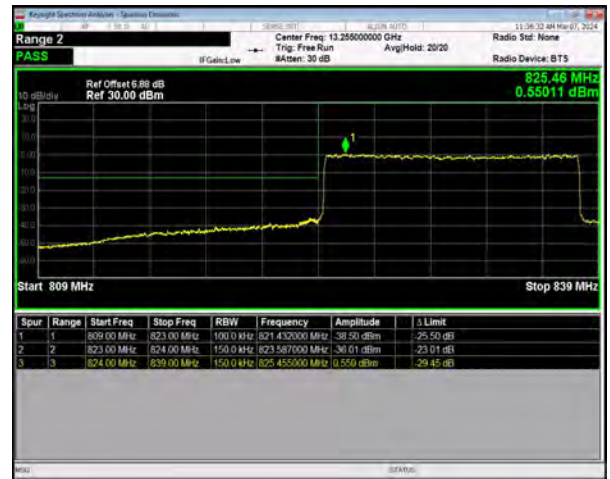
n5 SCS=15kHz DFT_64QAM BW=15MHz LowChannel=166300 RB=75@0
