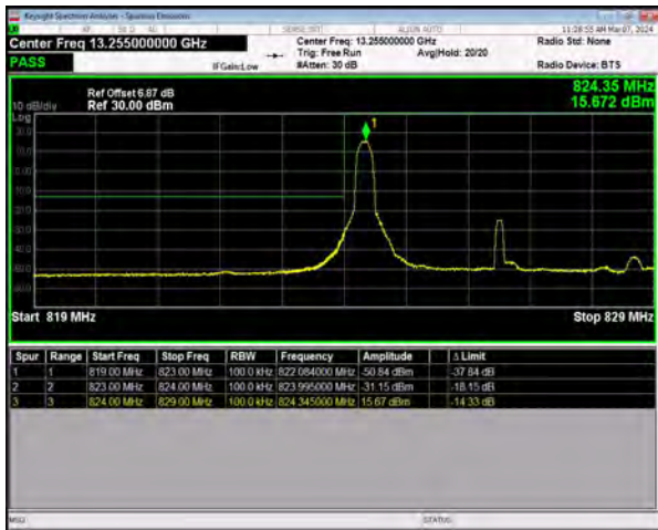
n5 SCS=15kHz DFT_256QAM BW=5MHz LowChannel=165300 RB=1@0
