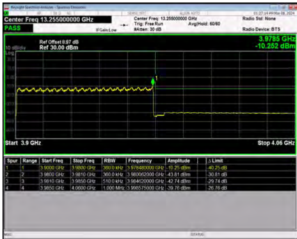
n77(3700-3980) SCS=30kHz DFT_16QAM BW=80MHz HighChannel=662666 RB=216@0
