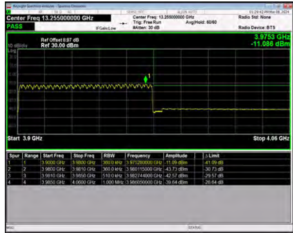
n77(3700-3980) SCS=30kHz CP_QPSK BW=80MHz HighChannel=662666 RB=217@0
