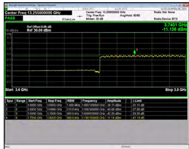
n77(3700-3980) SCS=30kHz DFT_QPSK BW=100MHz LowChannel=650000 RB=270@0
