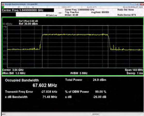
n77(3700-3980) SCS=30kHz CP_256QAM BW=70MHz Channel=656000 RB=189@0
