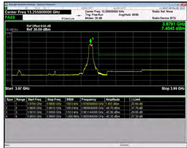
n77(3700-3980) SCS=30kHz DFT_16QAM BW=10MHz HighChannel=665000 RB=1@23
