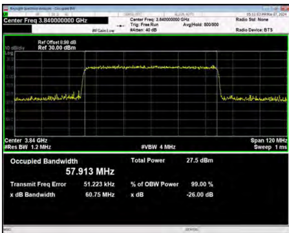
n77(3700-3980) SCS=30kHz CP_64QAM BW=60MHz Channel=656000 RB=162@0
