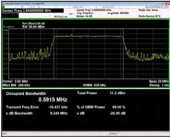
n77(3700-3980) SCS=30kHz DFT_BPSK BW=10MHz Channel=656000 RB=24@0
