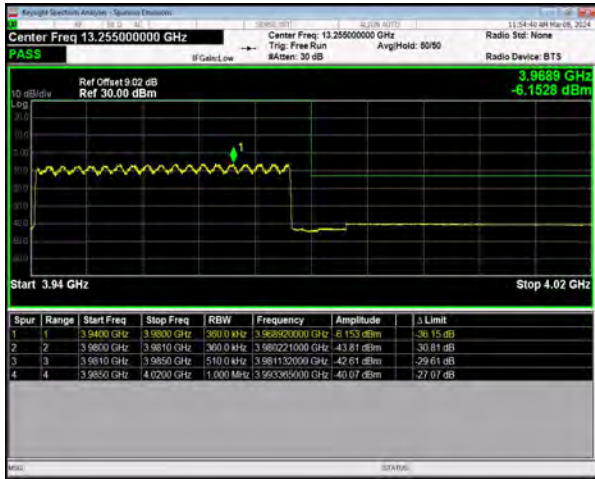
n77(3700-3980) SCS=30kHz DFT_BPSK BW=40MHz HighChannel=664000 RB=100@0
