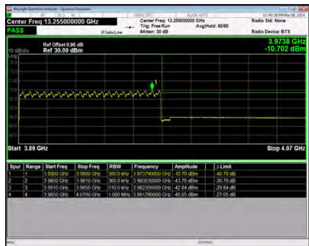
n77(3700-3980) SCS=30kHz CP_QPSK BW=90MHz HighChannel=662332 RB=245@0
