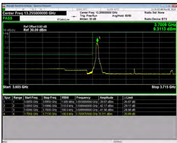
n77(3700-3980) SCS=30kHz DFT_BPSK BW=15MHz LowChannel=647168 RB=1@0
