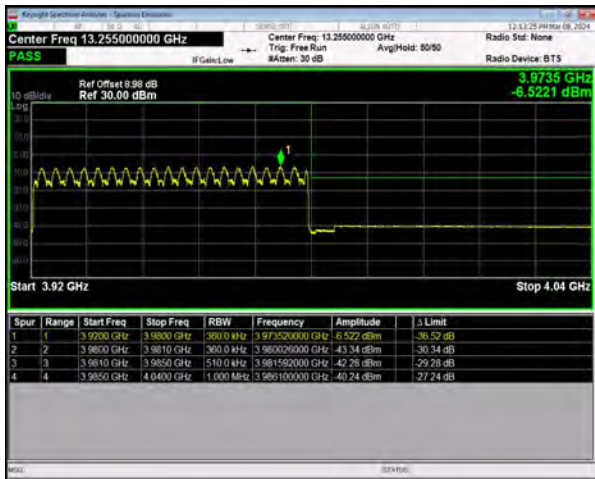
n77(3700-3980) SCS=30kHz DFT_BPSK BW=60MHz HighChannel=663332 RB=162@0
