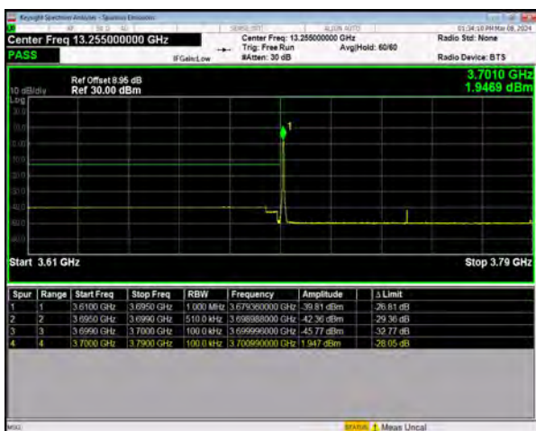
n77(3700-3980) SCS=30kHz DFT_256QAM BW=90MHz LowChannel=649668 RB=1@0
