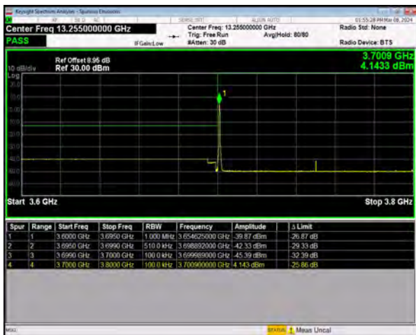
n77(3700-3980) SCS=30kHz DFT_256QAM BW=100MHz LowChannel=650000 RB=1@0
