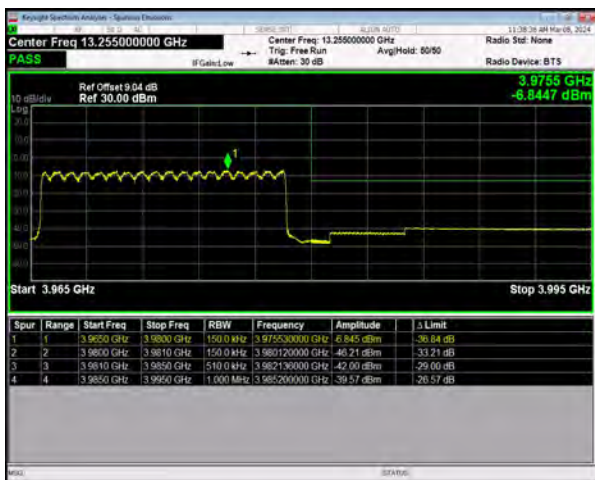
n77(3700-3980) SCS=30kHz DFT_64QAM BW=15MHz HighChannel=664832 RB=36@0
