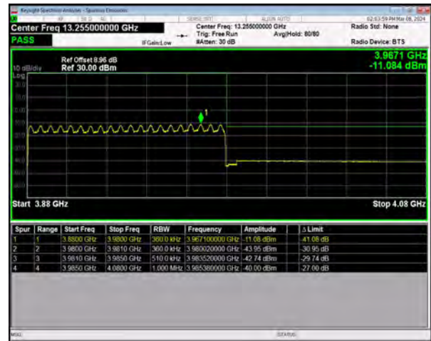
n77(3700-3980) SCS=30kHz CP_QPSK BW=100MHz HighChannel=662000 RB=273@0
