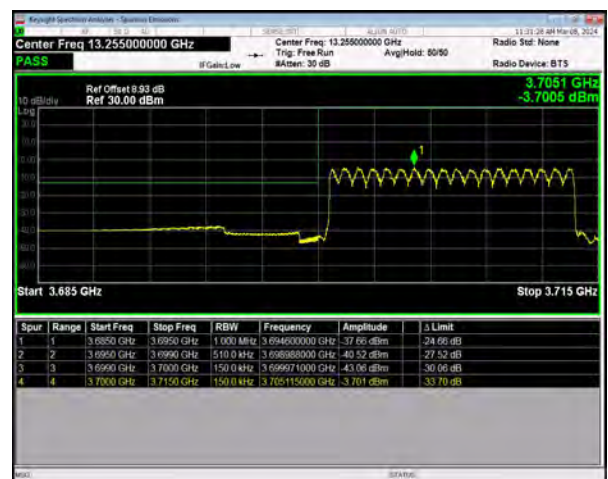
n77(3700-3980) SCS=30kHz DFT_BPSK BW=15MHz LowChannel=647168 RB=36@0
