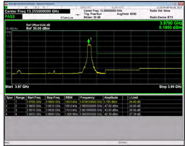
n77(3700-3980) SCS=30kHz DFT_256QAM BW=10MHz HighChannel=665000 RB=1@23
