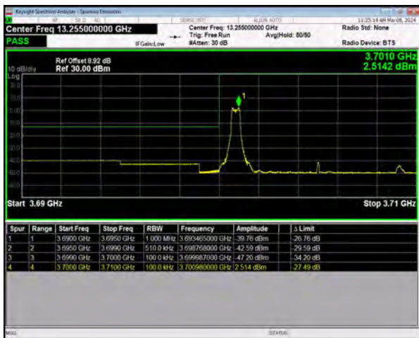
n77(3700-3980) SCS=30kHz DFT_256QAM BW=10MHz LowChannel=647000 RB=1@0
