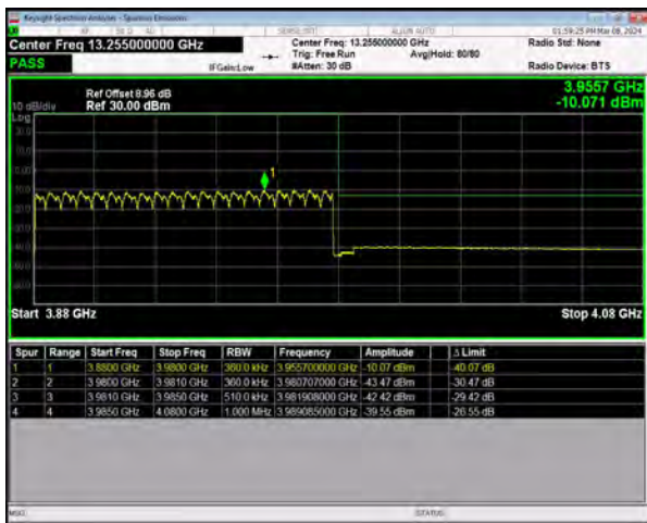
n77(3700-3980) SCS=30kHz DFT_QPSK BW=100MHz HighChannel=662000 RB=270@0
