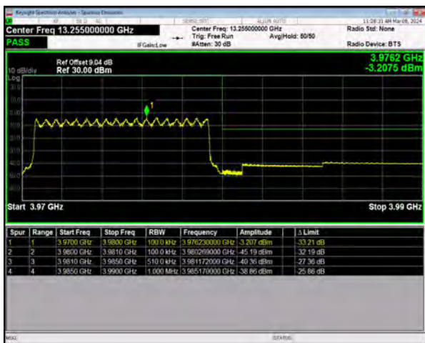
n77(3700-3980) SCS=30kHz DFT_16QAM BW=10MHz HighChannel=665000 RB=24@0
