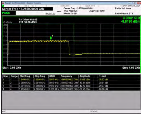
n77(3700-3980) SCS=30kHz DFT_64QAM BW=40MHz HighChannel=664000 RB=100@0
