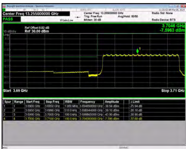
n77(3700-3980) SCS=30kHz CP_QPSK BW=10MHz LowChannel=647000 RB=24@0
