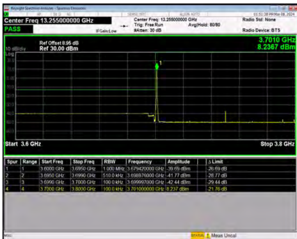
n77(3700-3980) SCS=30kHz DFT_QPSK BW=100MHz LowChannel=650000 RB=1@0
