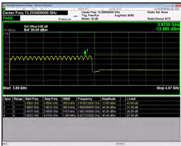
n77(3700-3980) SCS=30kHz DFT_256QAM BW=90MHz HighChannel=662332 RB=240@0
