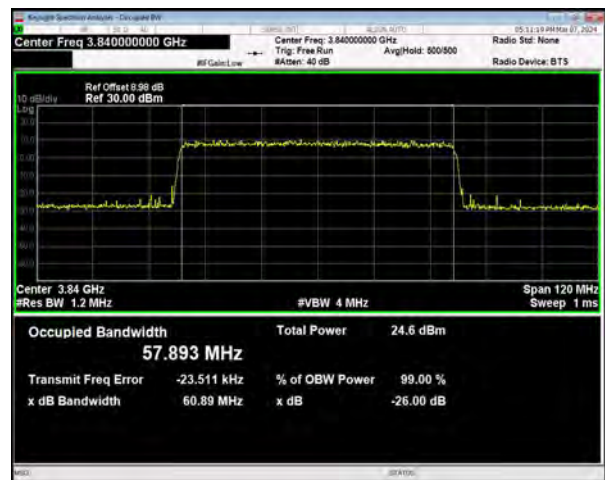
n77(3700-3980) SCS=30kHz CP_256QAM BW=60MHz Channel=656000 RB=162@0
