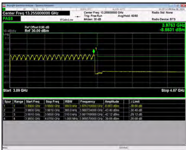
n77(3700-3980) SCS=30kHz DFT_QPSK BW=90MHz HighChannel=662332 RB=240@0
