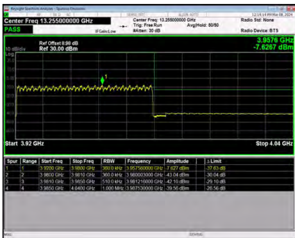
n77(3700-3980) SCS=30kHz DFT_QPSK BW=60MHz HighChannel=663332 RB=162@0
