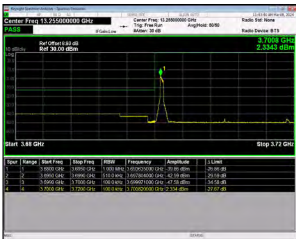
n77(3700-3980) SCS=30kHz DFT_256QAM BW=20MHz LowChannel=647334 RB=1@0
