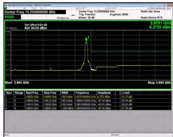
n77(3700-3980) SCS=30kHz DFT_256QAM BW=15MHz HighChannel=664832 RB=1@37
