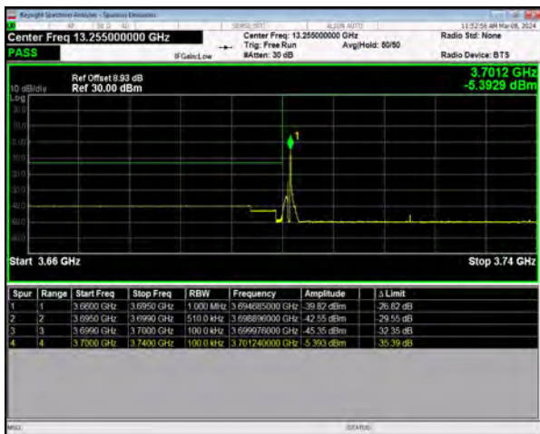
n77(3700-3980) SCS=30kHz DFT_256QAM BW=40MHz LowChannel=648000 RB=1@0
