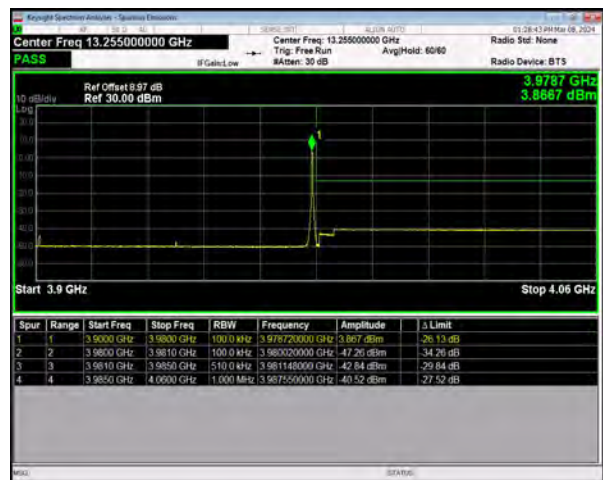
n77(3700-3980) SCS=30kHz DFT_256QAM BW=80MHz HighChannel=662666 RB=1@216
