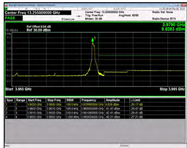
n77(3700-3980) SCS=30kHz DFT_BPSK BW=15MHz HighChannel=664832 RB=1@37
