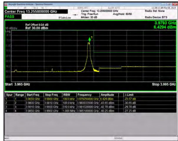
n77(3700-3980) SCS=30kHz DFT_64QAM BW=15MHz HighChannel=664832 RB=1@37
