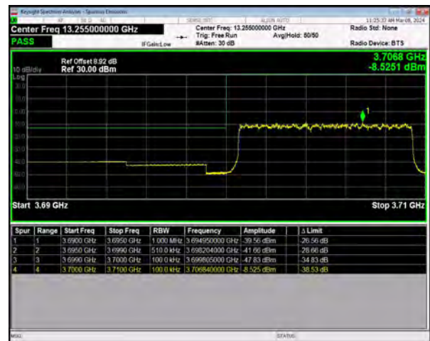
n77(3700-3980) SCS=30kHz DFT_256QAM BW=10MHz LowChannel=647000 RB=24@0
