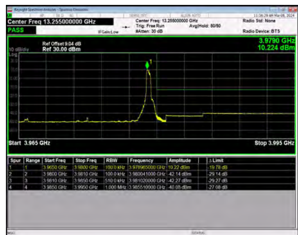
n77(3700-3980) SCS=30kHz DFT_QPSK BW=15MHz HighChannel=664832 RB=1@37
