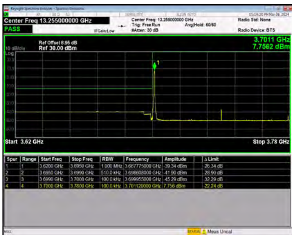
n77(3700-3980) SCS=30kHz DFT_BPSK BW=80MHz LowChannel=649334 RB=1@0
