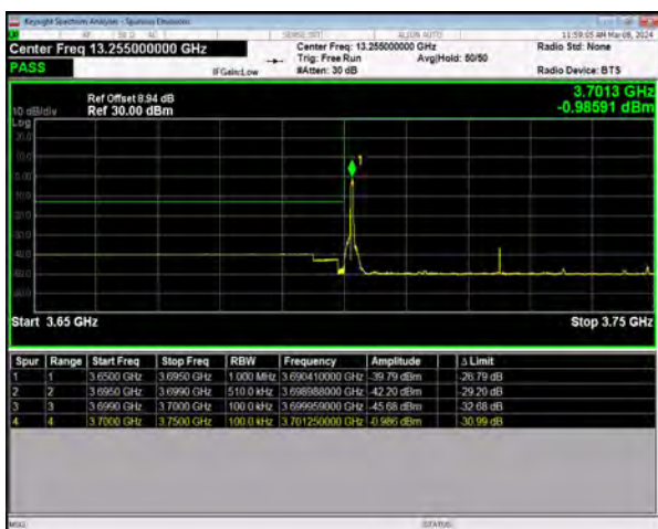
n77(3700-3980) SCS=30kHz DFT_BPSK BW=50MHz LowChannel=648334 RB=1@0
