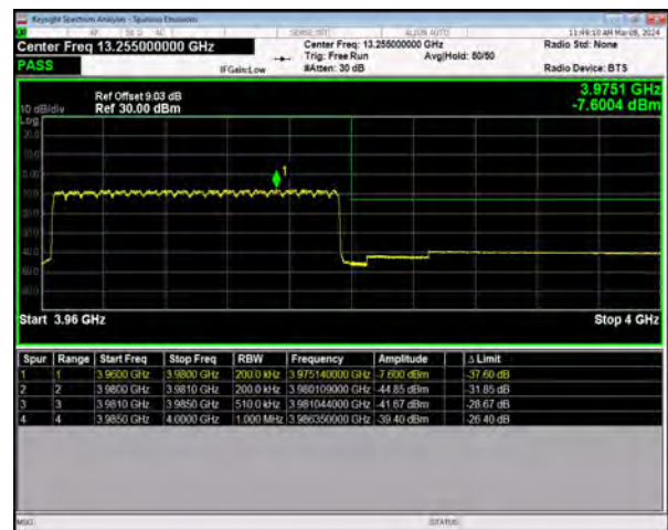
n77(3700-3980) SCS=30kHz CP_QPSK BW=20MHz HighChannel=664666 RB=51@0
