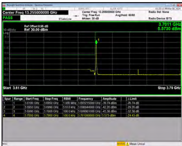
n77(3700-3980) SCS=30kHz DFT_64QAM BW=90MHz LowChannel=649668 RB=1@0
