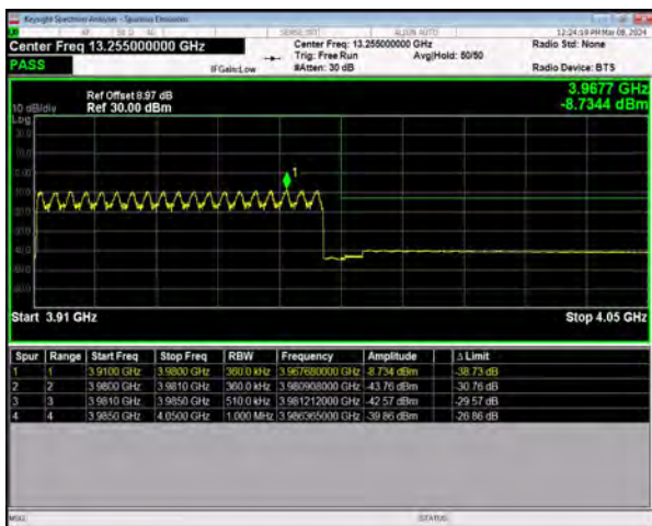
n77(3700-3980) SCS=30kHz DFT_16QAM BW=70MHz HighChannel=663000 RB=180@0
