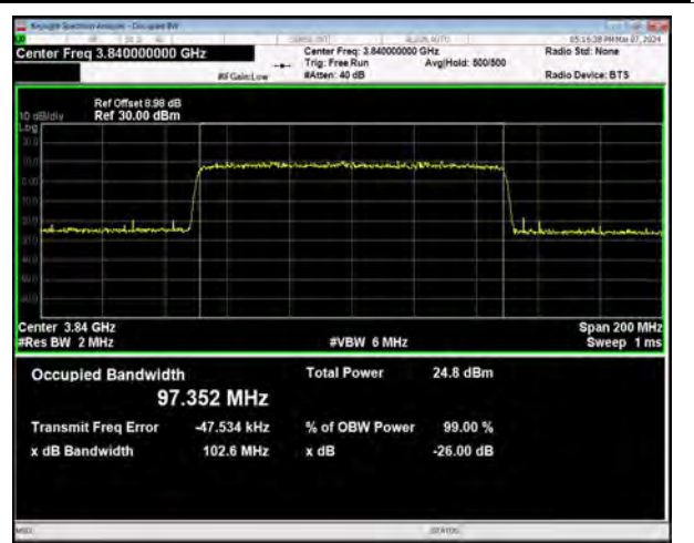
n77(3700-3980) SCS=30kHz CP_256QAM BW=100MHz Channel=656000 RB=273@0
