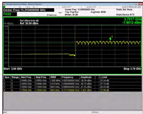
n77(3700-3980) SCS=30kHz DFT_QPSK BW=60MHz LowChannel=648668 RB=162@0
