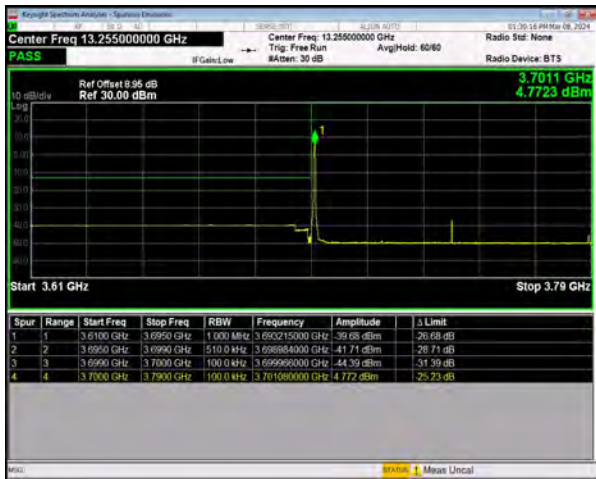
n77(3700-3980) SCS=30kHz DFT_BPSK BW=90MHz LowChannel=649668 RB=1@0
