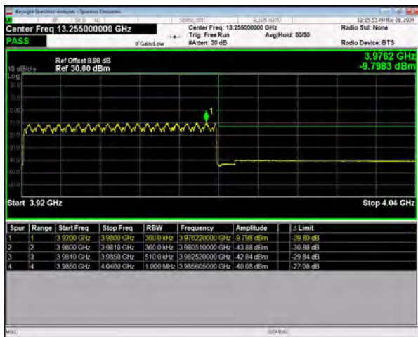
n77(3700-3980) SCS=30kHz DFT_64QAM BW=60MHz HighChannel=663332 RB=162@0
