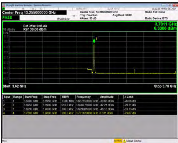
n77(3700-3980) SCS=30kHz DFT_64QAM BW=80MHz LowChannel=649334 RB=1@0
