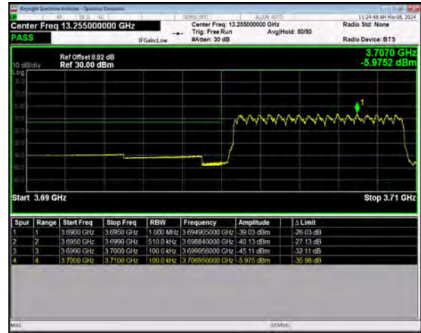
n77(3700-3980) SCS=30kHz DFT_64QAM BW=10MHz LowChannel=647000 RB=24@0
