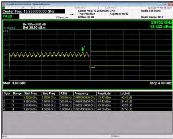
n77(3700-3980) SCS=30kHz DFT_256QAM BW=100MHz HighChannel=662000 RB=270@0
