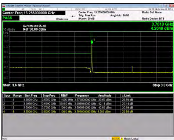
n77(3700-3980) SCS=30kHz DFT_16QAM BW=100MHz LowChannel=650000 RB=1@0
