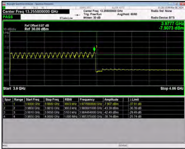
n77(3700-3980) SCS=30kHz DFT_QPSK BW=80MHz HighChannel=662666 RB=216@0
