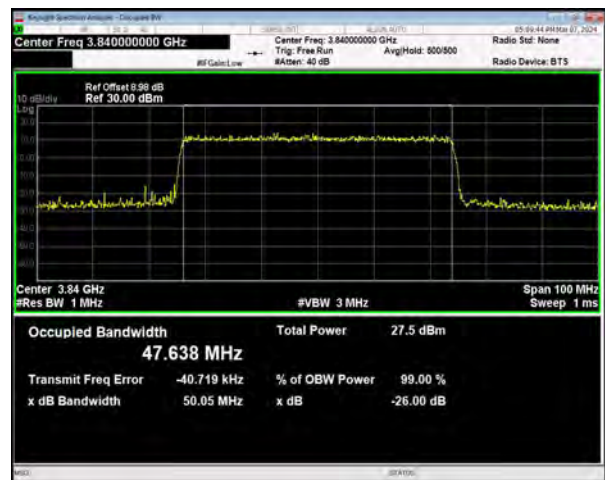
n77(3700-3980) SCS=30kHz CP_64QAM BW=50MHz Channel=656000 RB=133@0
