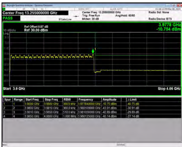
n77(3700-3980) SCS=30kHz DFT_64QAM BW=80MHz HighChannel=662666 RB=216@0
