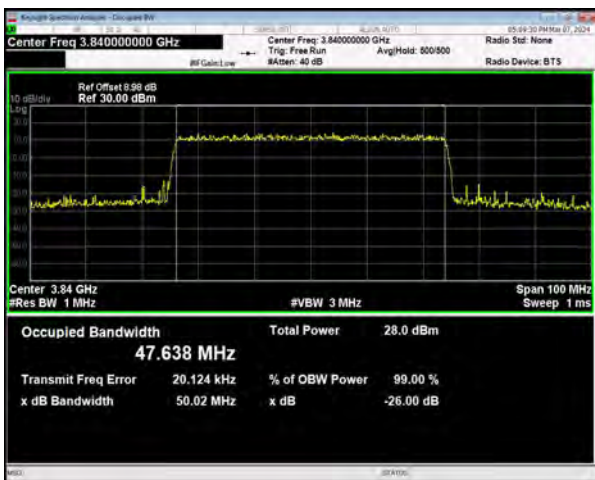
n77(3700-3980) SCS=30kHz CP_16QAM BW=50MHz Channel=656000 RB=133@0
