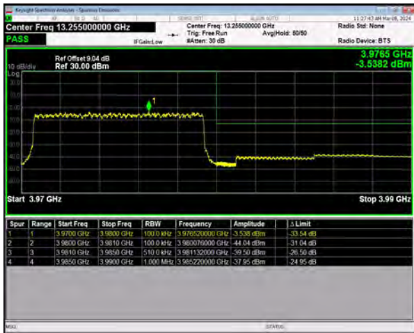
n77(3700-3980) SCS=30kHz DFT_QPSK BW=10MHz HighChannel=665000 RB=24@0
