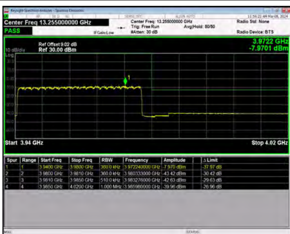
n77(3700-3980) SCS=30kHz DFT_16QAM BW=40MHz HighChannel=664000 RB=100@0
