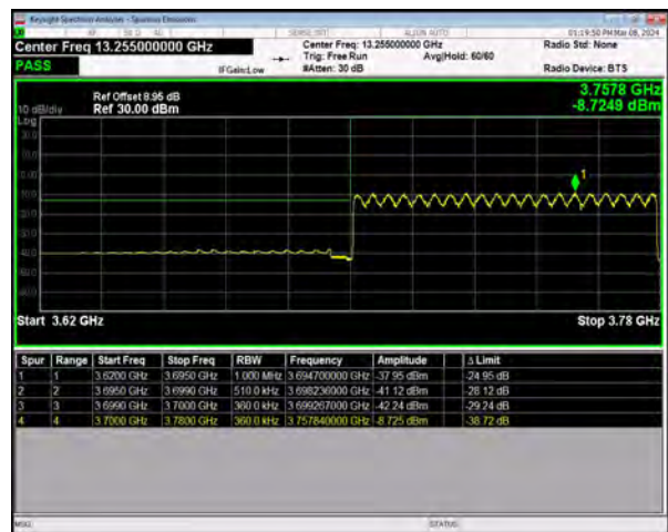
n77(3700-3980) SCS=30kHz DFT_BPSK BW=80MHz LowChannel=649334 RB=216@0
