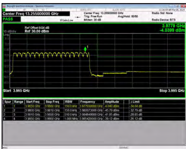
n77(3700-3980) SCS=30kHz DFT_BPSK BW=15MHz HighChannel=664832 RB=36@0
