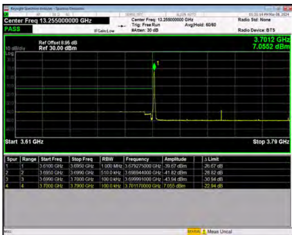
n77(3700-3980) SCS=30kHz DFT_QPSK BW=90MHz LowChannel=649668 RB=1@0
