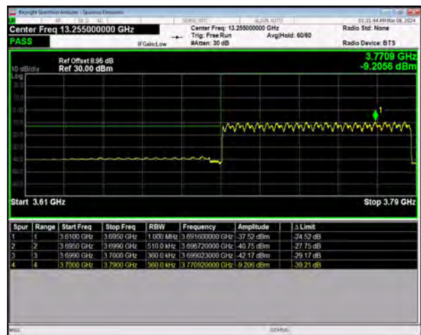
n77(3700-3980) SCS=30kHz DFT_QPSK BW=90MHz LowChannel=649668 RB=240@0
