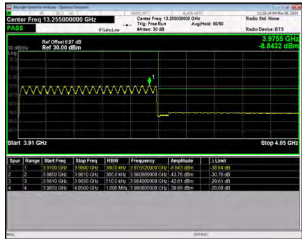
n77(3700-3980) SCS=30kHz CP_QPSK BW=70MHz HighChannel=663000 RB=189@0
