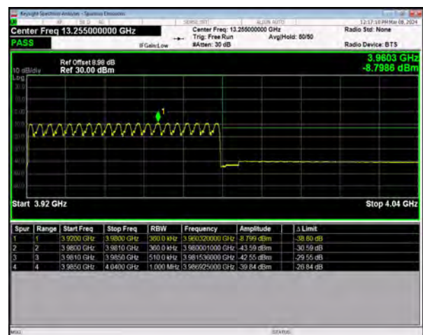
n77(3700-3980) SCS=30kHz CP_QPSK BW=60MHz HighChannel=663332 RB=162@0
