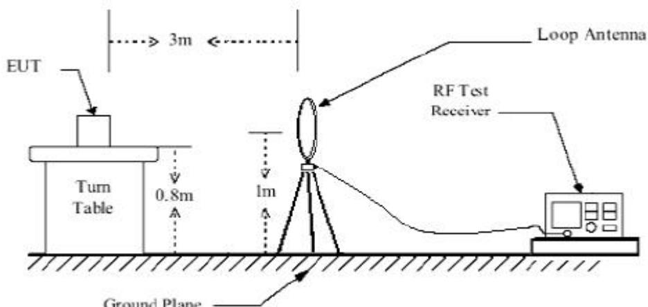
For radiated test from 30MHz to 1GHz
