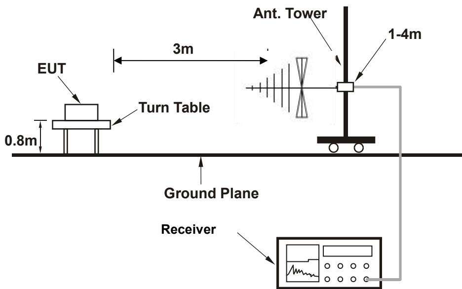
For radiated test from 1GHz to 18GHz
