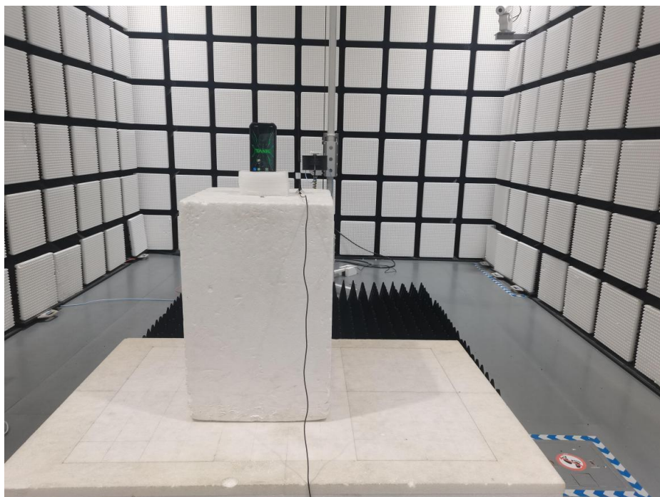
Radiated spurious emission Test Setup-2(Above 1GHz)
