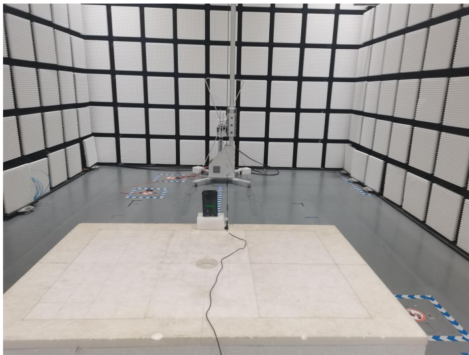
Radiated spurious emission Test Setup-2(Above 1GHz)
