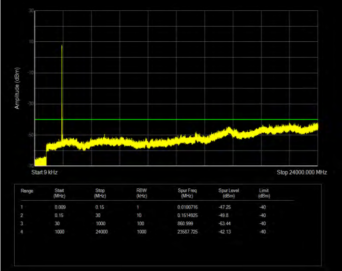
Band40(2305-2315) 16QAM BW=5MHz Channel=38725 RB Size=25 Position=#0
