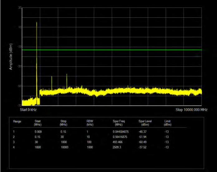
Band26(824-849) QPSK BW=5MHz Channel=27015 RB Size=25 Position=#0
