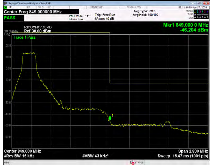
Band5 16QAM BW=1.4MHz Channel=20643 RB Size=1 Position=#0
