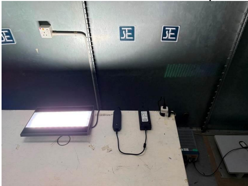
Measurement of Conducted Emission Test Set Up
