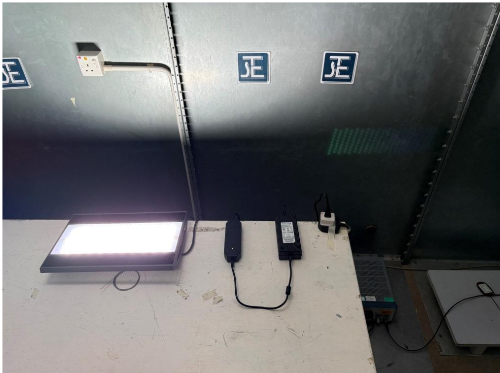
Measurement of Conducted Emission Test Set Up
