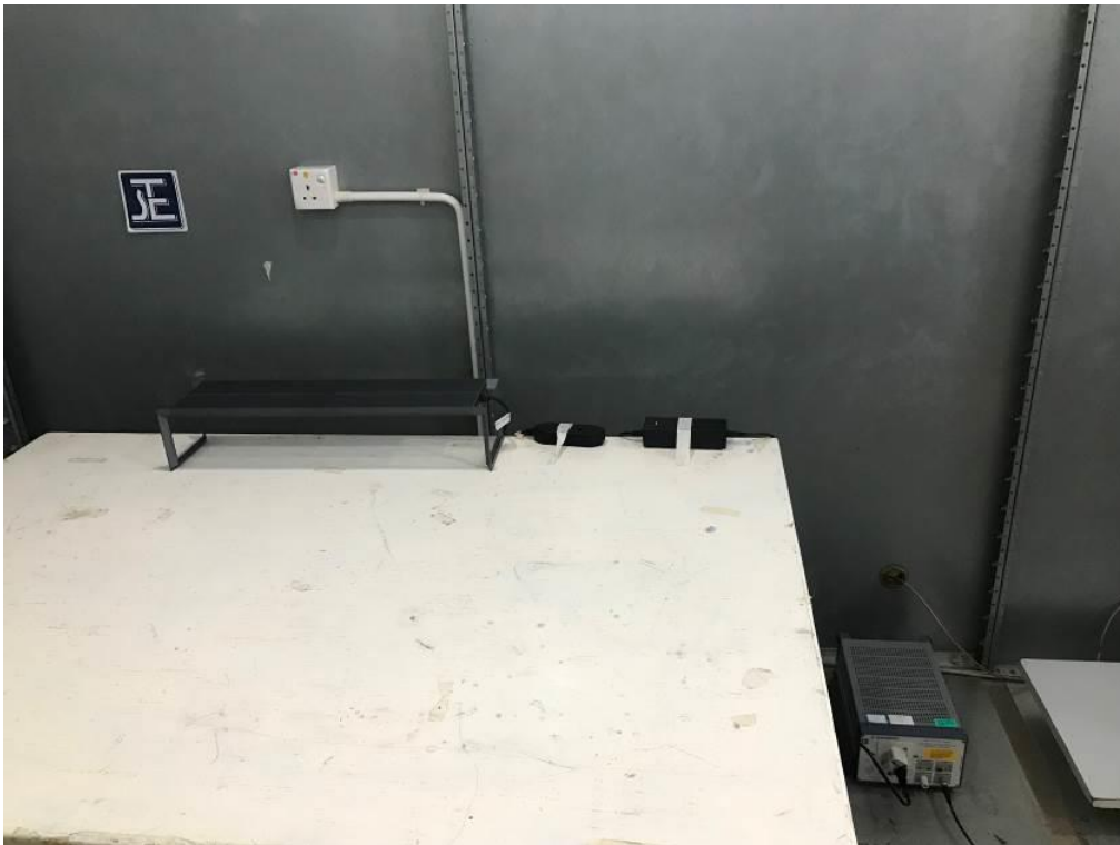
Measurement of Conducted Emission Test Set Up
