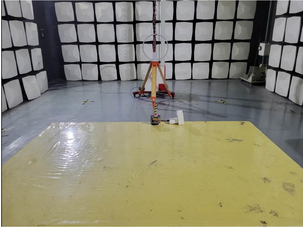
Test Photo Radiated emission (Below 30MHz)
