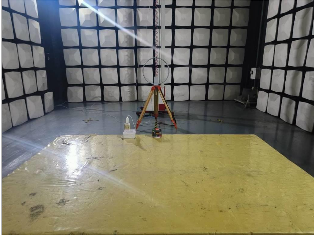
Test Photo Radiated emission (Below 30MHz)
