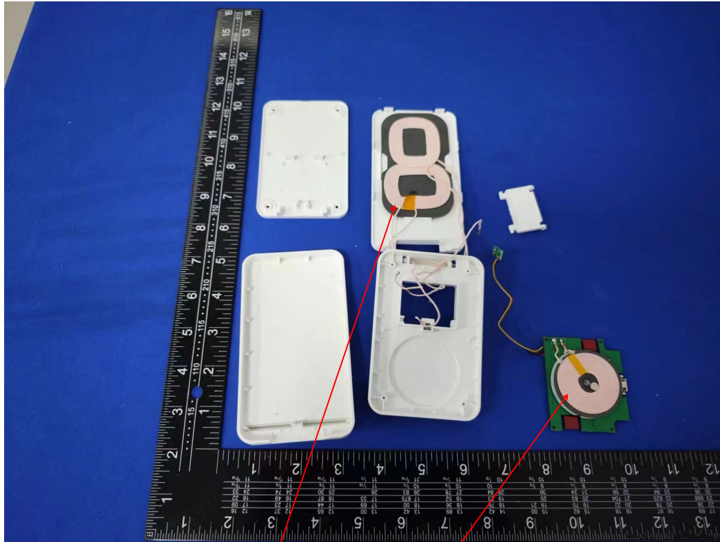
Inductive Loop Antenna
