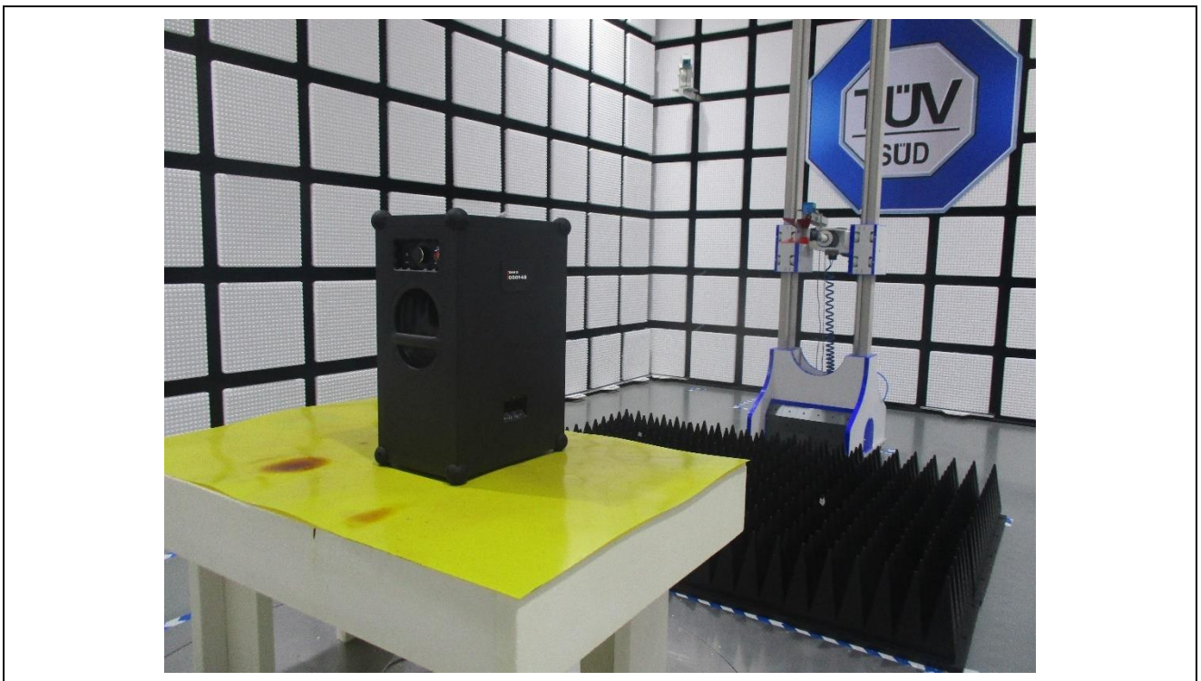
Radiated Emission test (1000MHz to 18000MHz)
