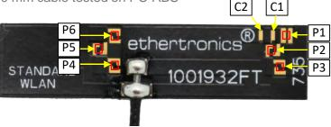
\*This antenna has unique features enabling limited range RF tuning by leaving P1 - P6 and C1 - C2 connected by "solder bridge" or disconnected with a "cut" to the trace. Refer to detailed tuning options below.
