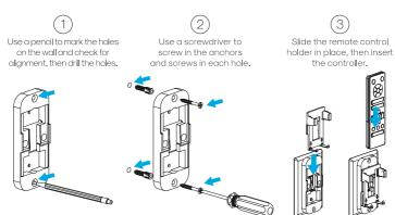
Alternatively, you can use the 3M sticker to fix the bracket on the wall.
