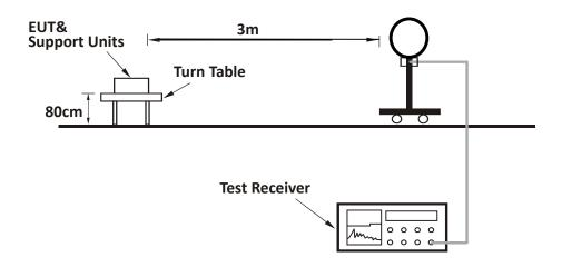
For Radiated emission 30MHz to 1GHz:
