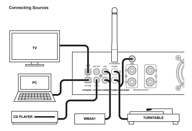
The HTA200 is capable of receiving signals directly from a wide variety of sources. Using high quality cables will ensure the best possible transmission from your connected devices.
