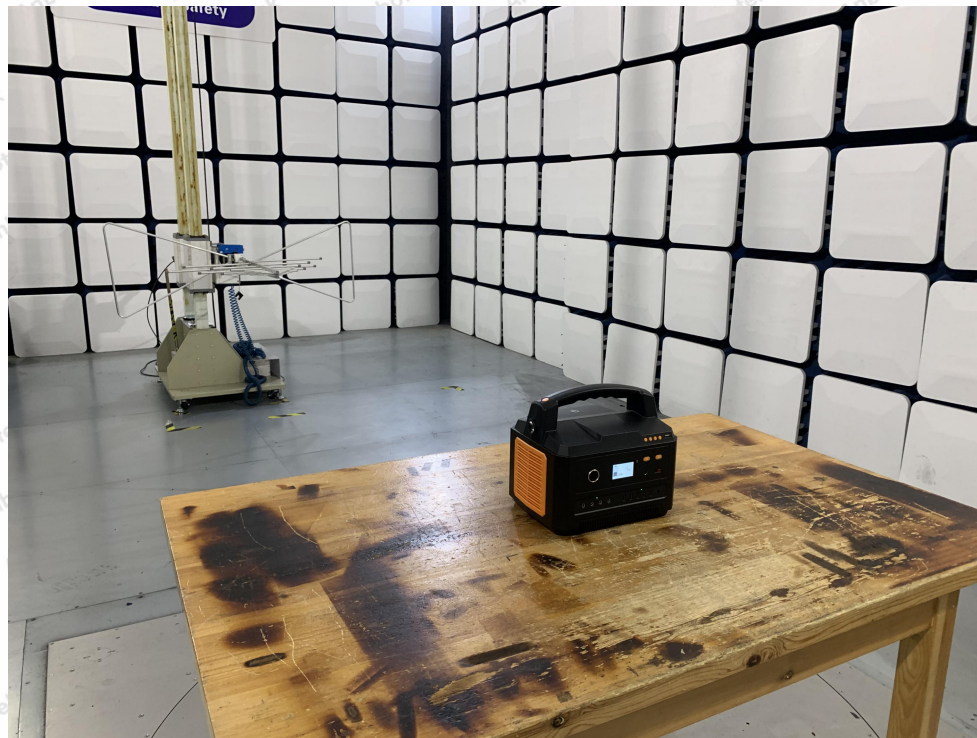
Photo of Radiation Emission Test
