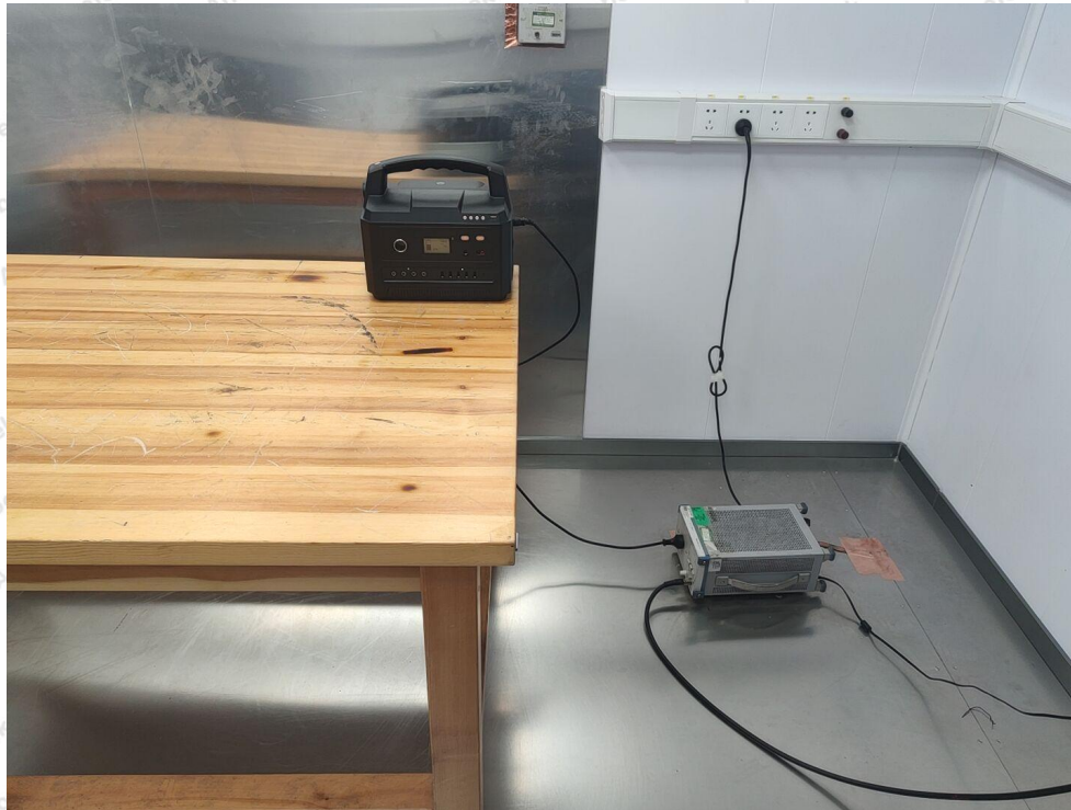
Photo of Conducted Emission Measurement
