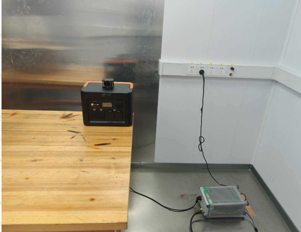
Photo of Conducted Emission Measurement
