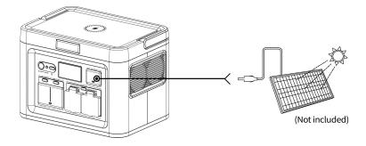
$\triangle$ The total open circuit voltage of solar modules after series-parallel connection should not exceed the specified voltage! please confirm the same voltage specification.
