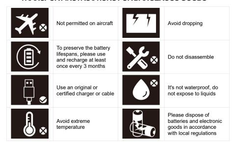
⚠ The H700 Series power station meets all legal requirements for the transportation of dangerous goods. The capacity of the lithium battery pack exceeds 100Wh. According to international standards, if the power station is transported by air, it must be transported in accordance with IATA standard packaging. The instructions and labeling requirements of the International Air Transport Association and related declarations must be completed.
