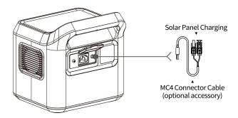
$\triangle$ The total open circuit voltage of solar modules after series-parallel connection should not exceed the specified voltage! please confirm the same voltage specification.
