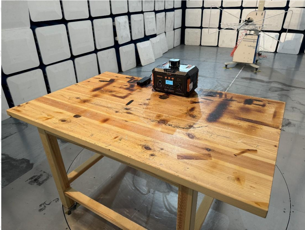
Photo of Radiation Emission Test (30MHz~1000MHz)
