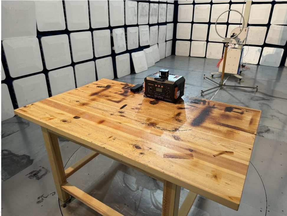
Photo of Radiation Emission Test (below 30MHz)
