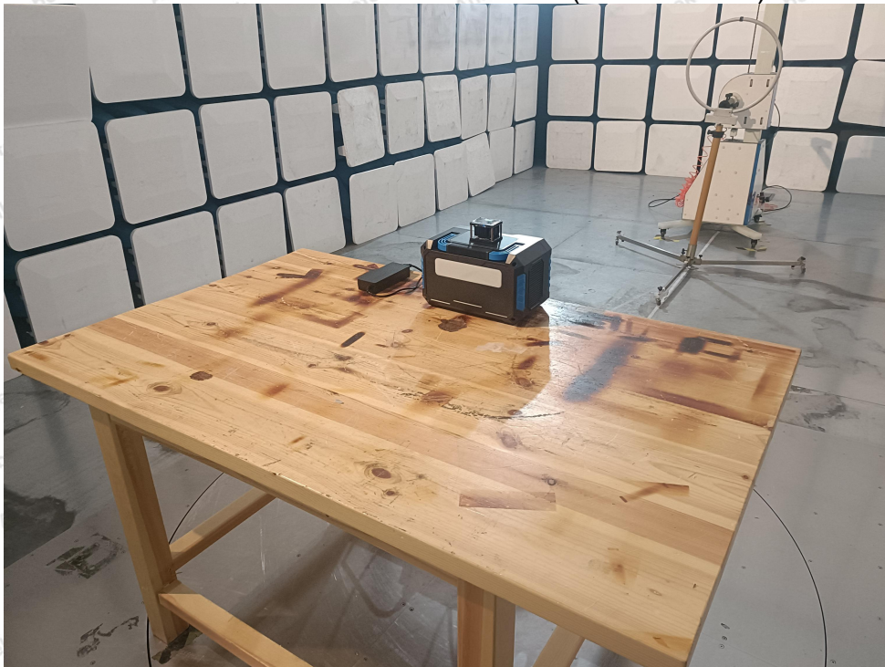
Photo of Radiation Emission Test (below 30MHz)
