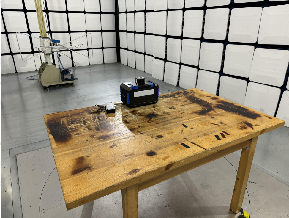
Photo of Radiation Emission Test (30MHz~1000MHz)
