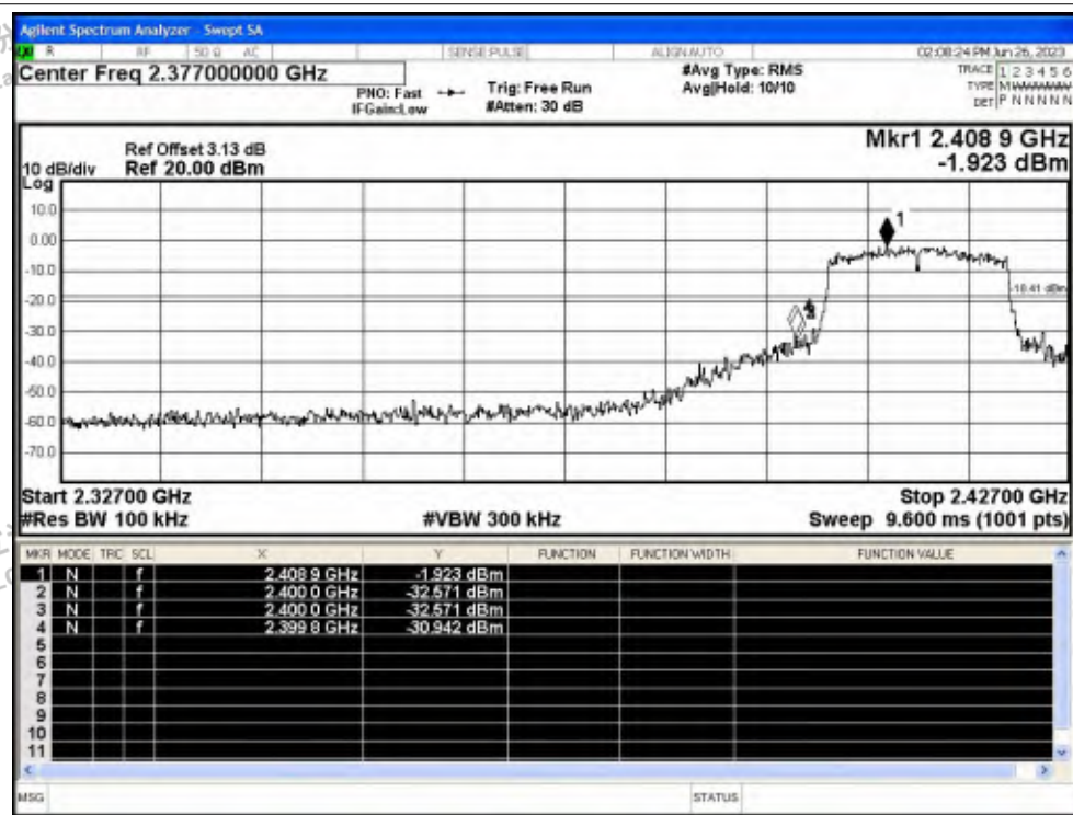
Band Edge NVNT n20 2412MHz Ant1 Emission
