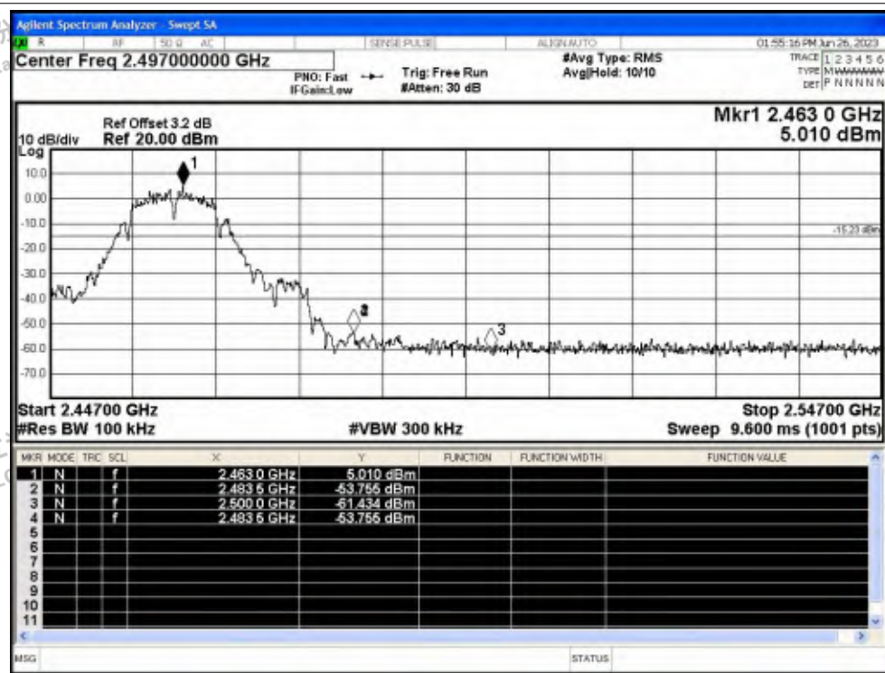
Band Edge NVNT b 2462MHz Ant1 Emission
