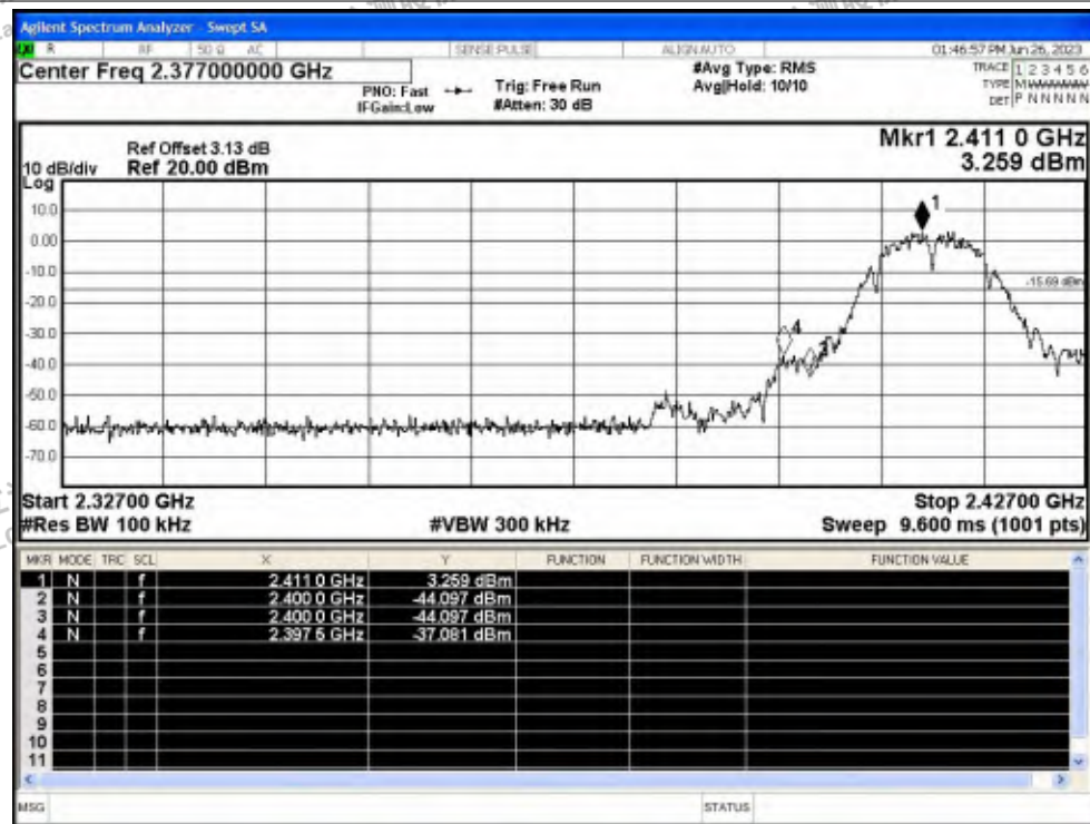
Band Edge NVNT b 2412MHz Ant1 Emission
