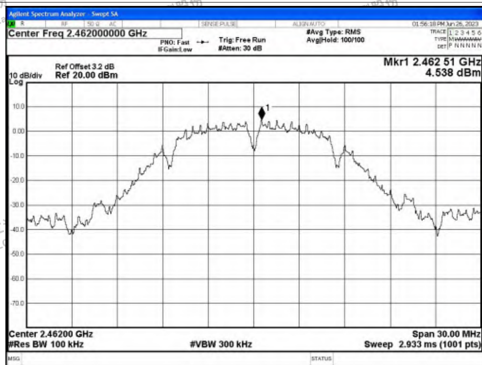
Tx. Spurious NVNT b 2462MHz Ant1 Emission
