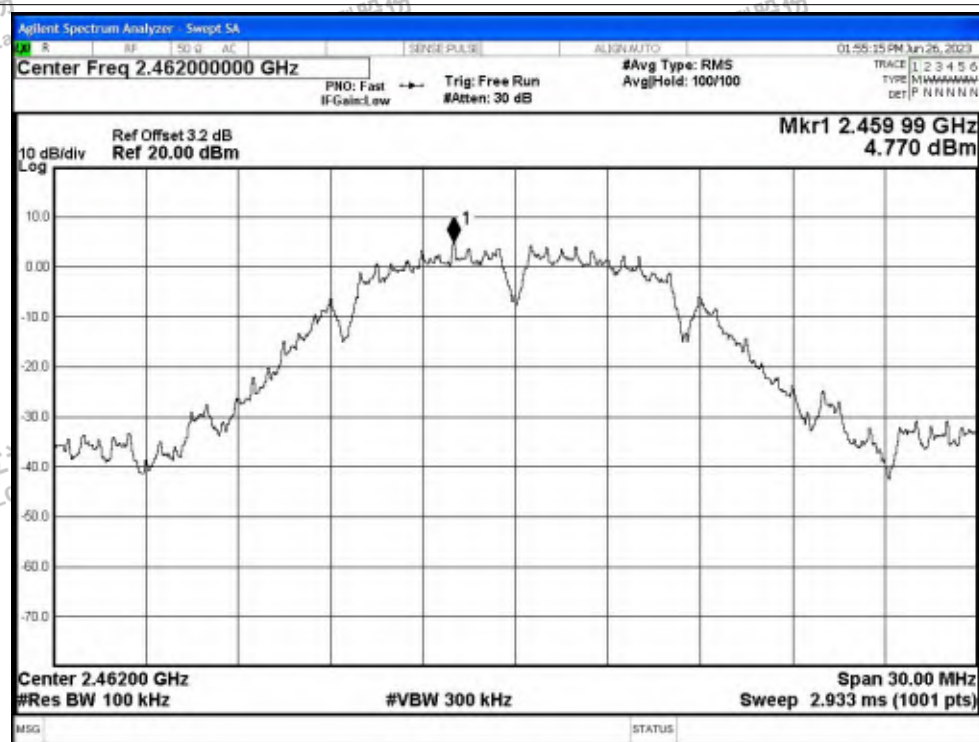
Band Edge NVNT b 2462MHz Ant1 Emission
