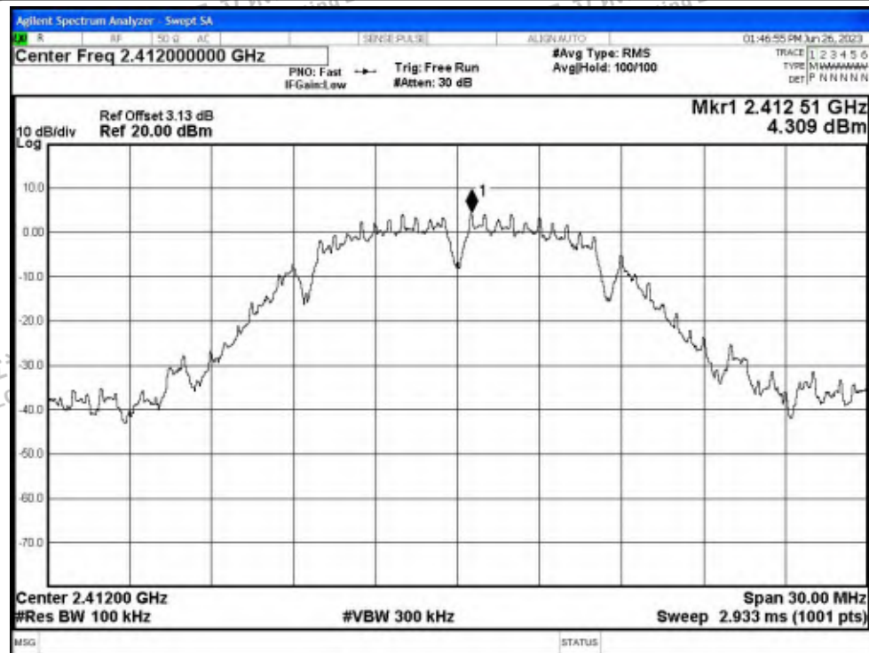
Band Edge NVNT b 2412MHz Ant1 Emission
