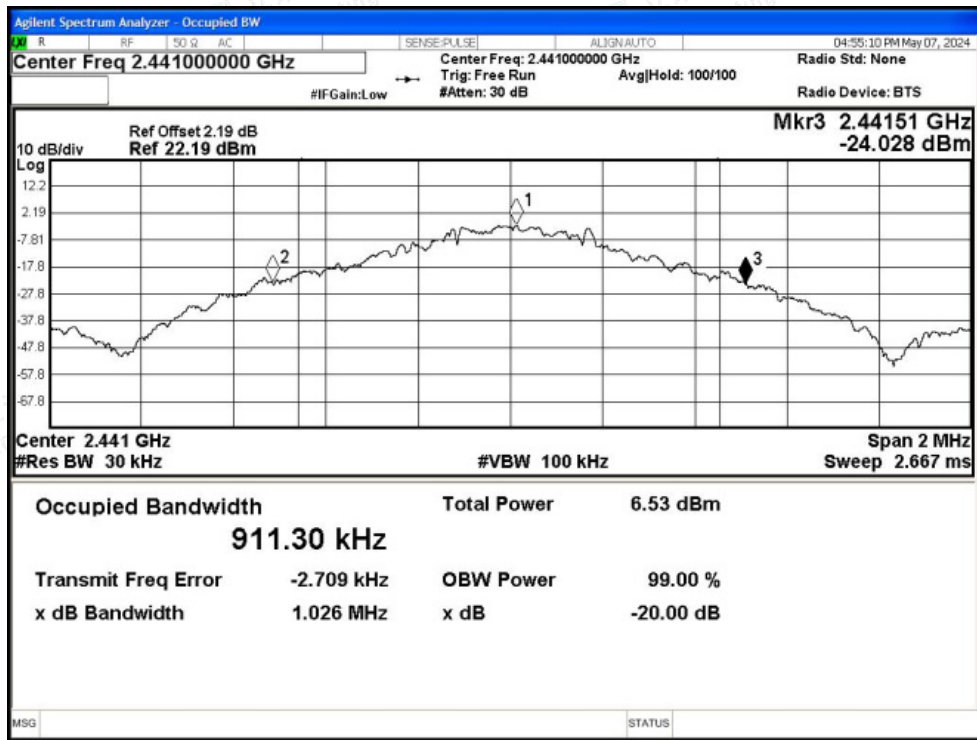
-20dB Bandwidth NVNT 1-DH5 2441MHz Ant1
