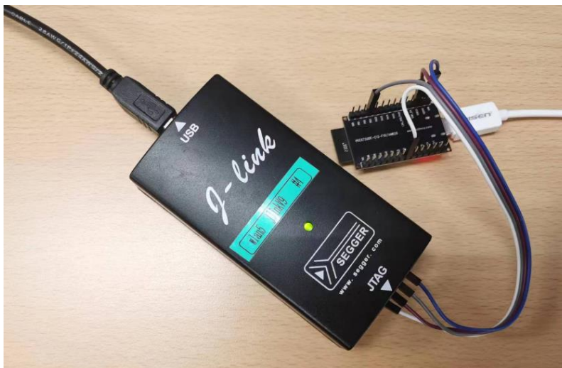
Fig 1-3 J-Link and Ameba-D SWD connection
