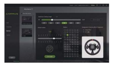
Enter the steering wheel interface and set the center of the steering wheel.
