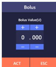
**(3)** When the value of bolus is greater than 0, the "Start" button (as shown in Figure A.5.2) will turn orange. Click "Start" to open the confirmation interface, then click "ACT" for the insulin pump controller to send a delivery instruction to the insulin pump. Click "ESC" to return to the Bolus
