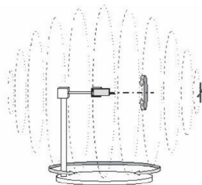
Figure (2) The three-dimensional positioning device of the mobile phone in the dark room
