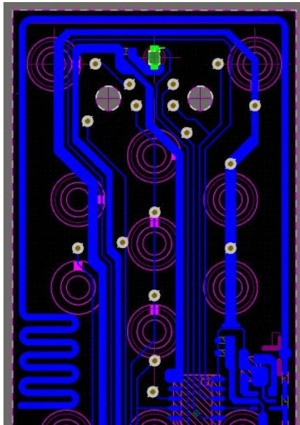
Antenna transmission frequency: 433.925MHz
