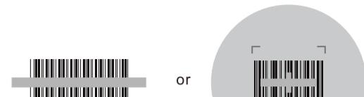
1. Press & hold Trigger, Illumination LED and Aiming LED cast an Illumination Pattern and an Aiming Pattern.
