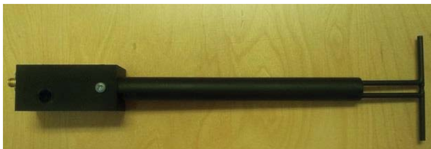
Figure 1 – MVG COMOSAR Validation Dipole
