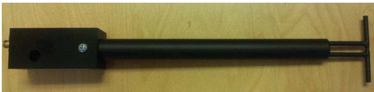
Figure 1 – MVG COMOSAR Validation Dipole
