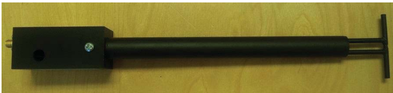
Figure 1 – MVG COMOSAR Validation Dipole
