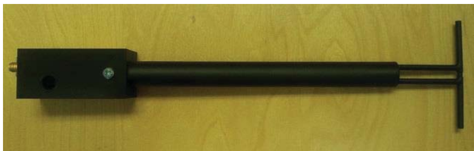
Figure 1 – MVG COMOSAR Validation Dipole
