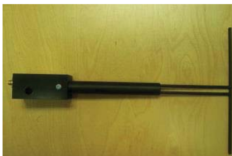
Figure 1 – MVG COMOSAR Validation Dipole
