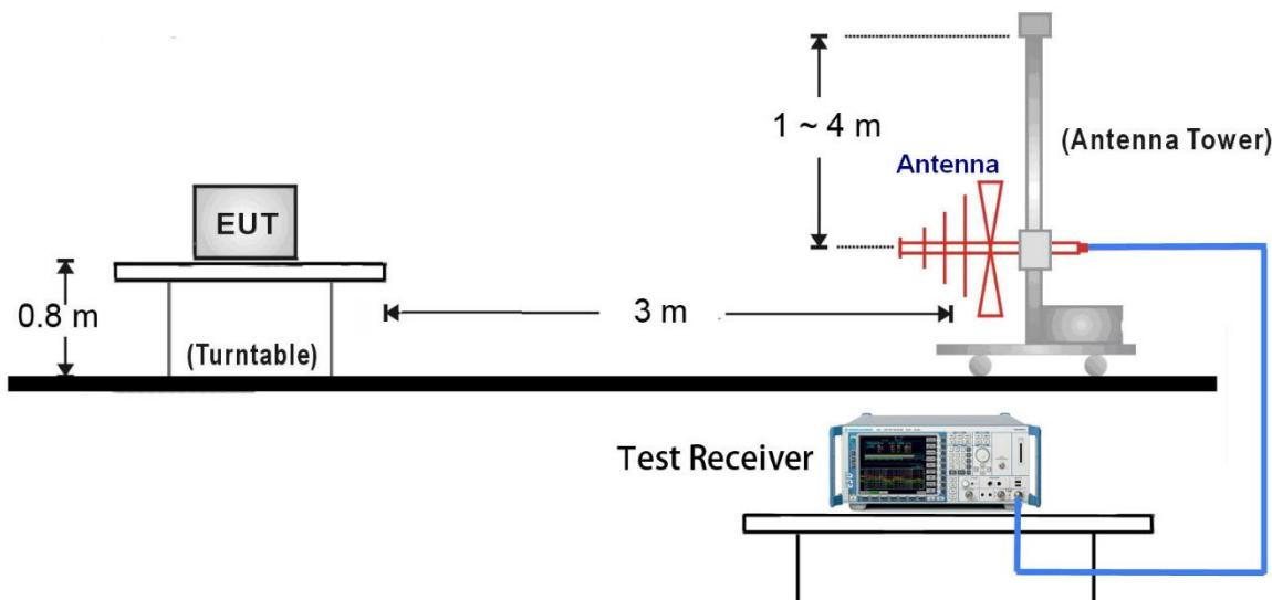
1GHz ~ 18GHz Test Setup:
