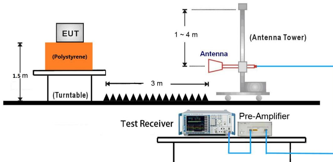
18GHz ~26.5GHz Test Setup:
