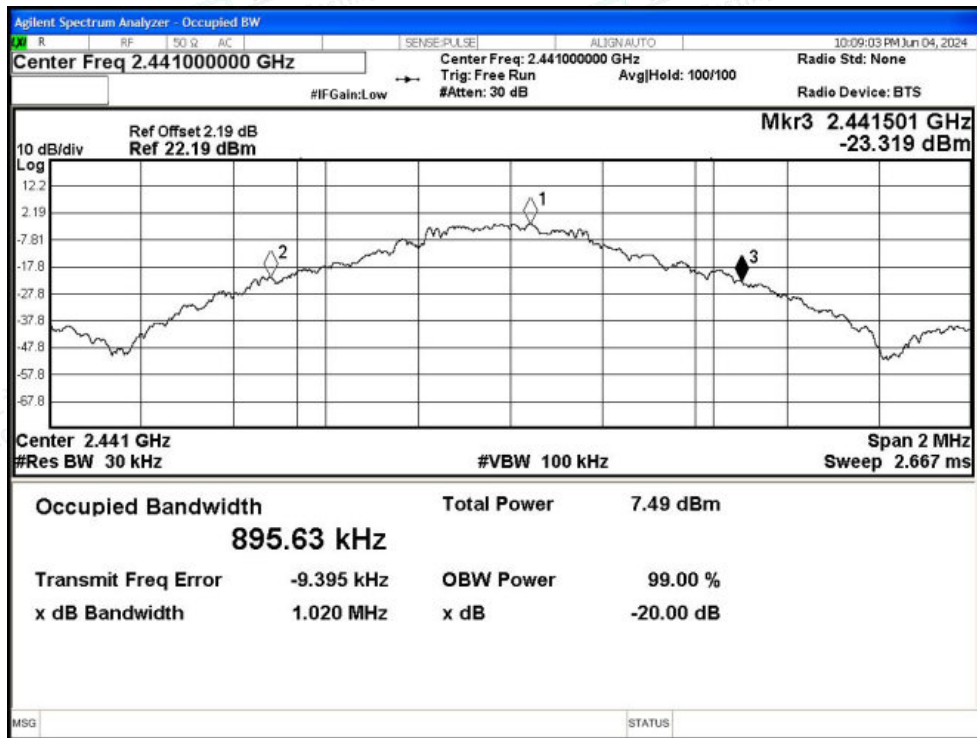
-20dB Bandwidth NVNT 1-DH5 2441MHz Ant1
