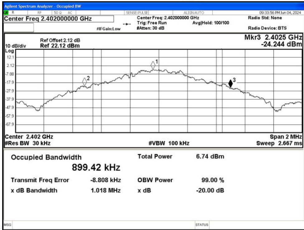
-20dB Bandwidth NVNT 1-DH5 2441MHz Ant1
