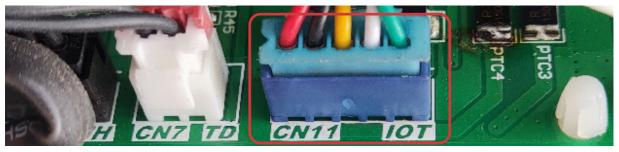
Power ON the condensing unit and check if the IoT device is working properly. The normal working state of IoT device should be the blue LED (No.1) is blinking with other LEDs light OFF.
