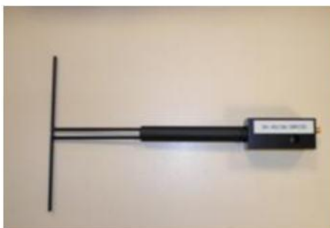
Figure 1 – Satimo COMOSAR Validation Dipole
