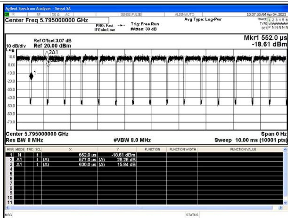
Duty Cycle NVNT ac80 5775MHz Ant1
