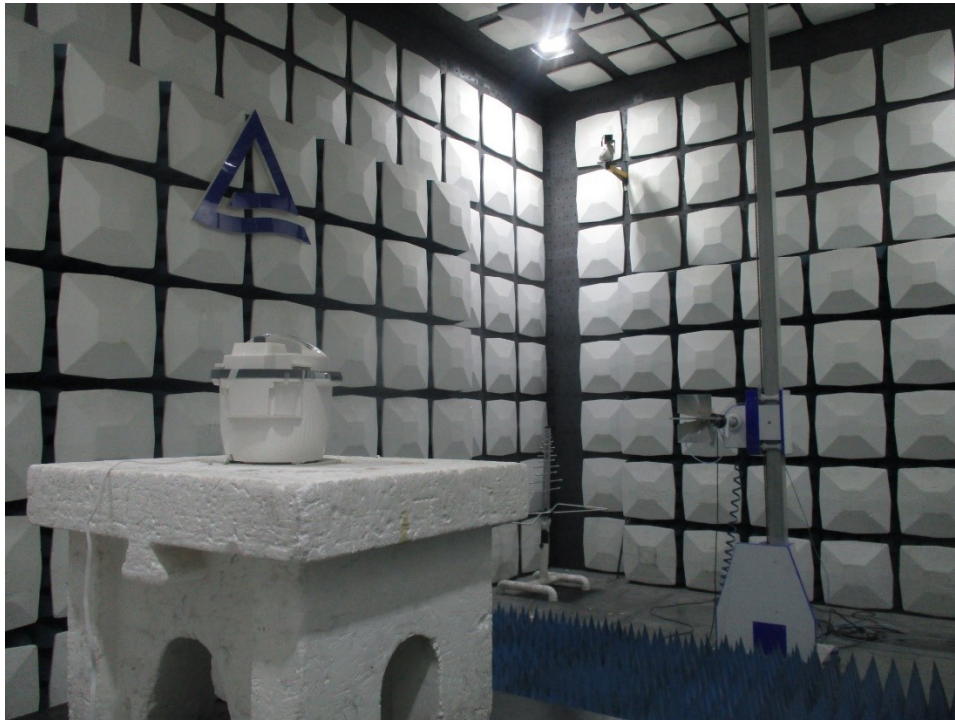
Photograph 3: Set-up photo for Radiated Spurious Emission, above 6GHz
