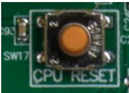
Figure 20-61: NET2-FFANN CPU Reset Pushbutton SW17
