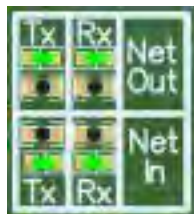
Figure 20-10: Network Activity LEDs
