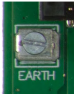
Figure 20-21: Earth/Ground connection point (K602)
