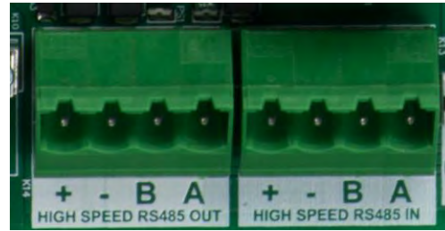
Figure 20-55: NET2-FFANN External Network Peripheral Bus connectors K14 and K13
