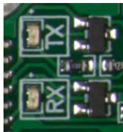
Figure 20-8: Network Input Connector LEDs
