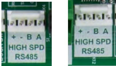
Figure 20-54: NET2-FFANN Internal Network Peripheral Bus connectors K4 and K12
