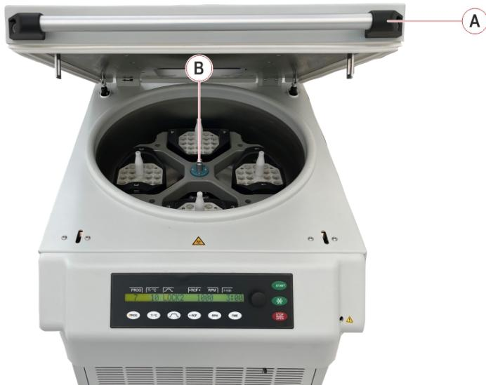
5. Remove all bucket inserts from the rotor (Figure 134 – B) and put them in safe place for inspection.
