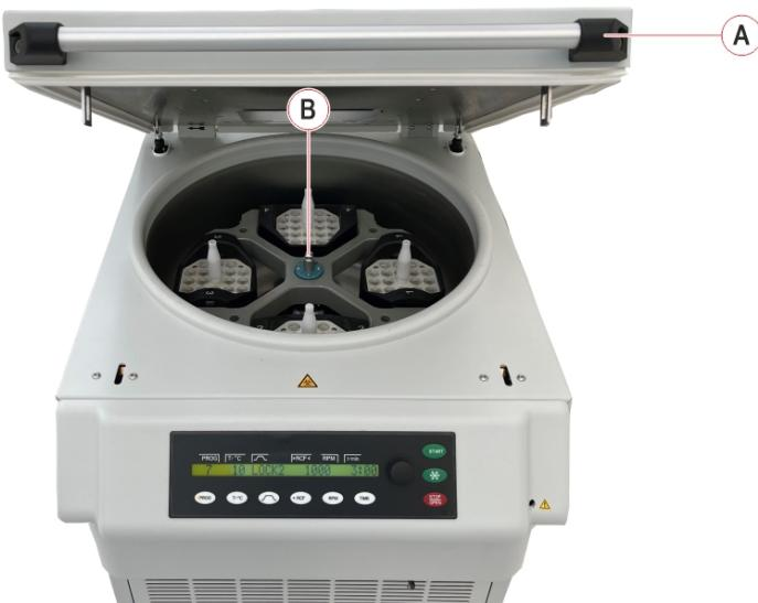
5. Remove all bucket inserts from the rotor ([Figure 139 – B](#)) and put them in safe place for the cleaning task.
