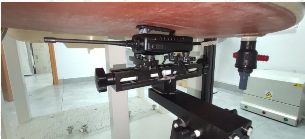
Body-worn, the front of the EUT towards ground (The distance was 0mm)
