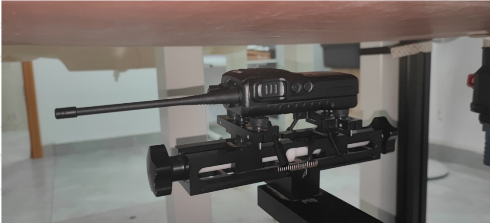
Face-held, the front of the EUT towards phantom (The distance was 25mm)
