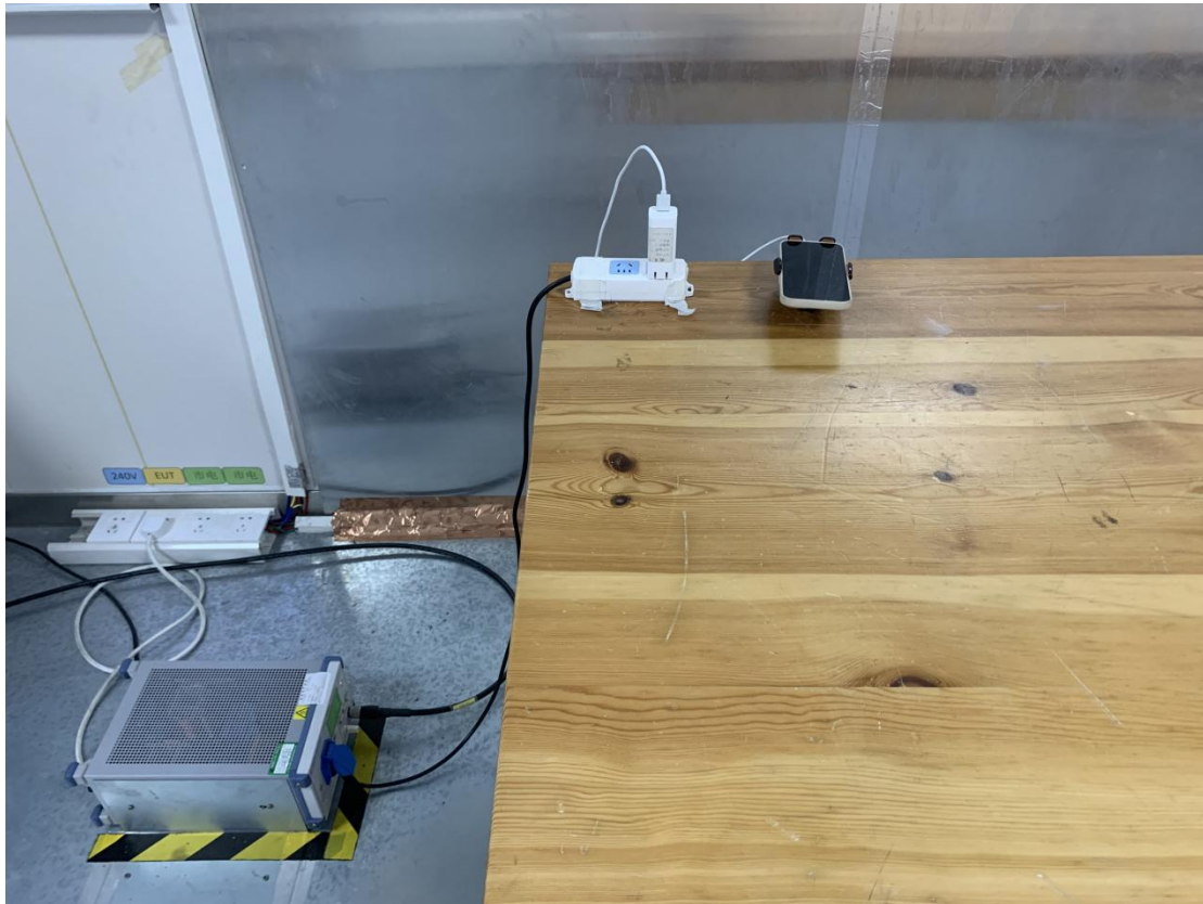
Conducted emission test setup
