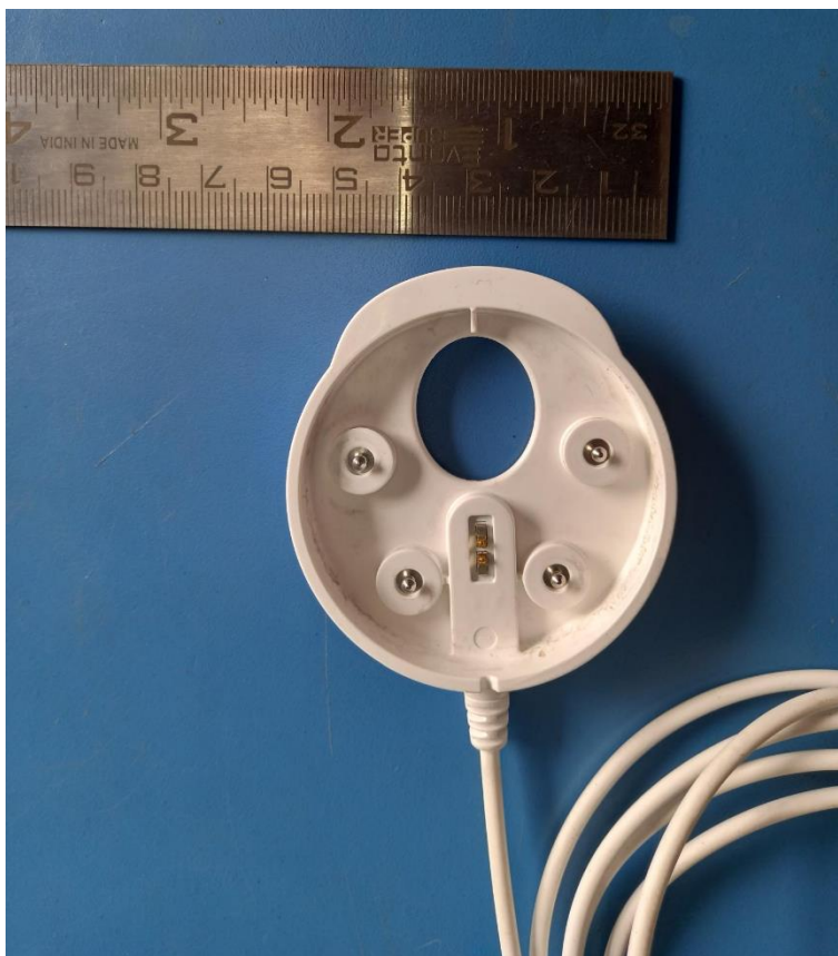
Docking station rear dimensional view
