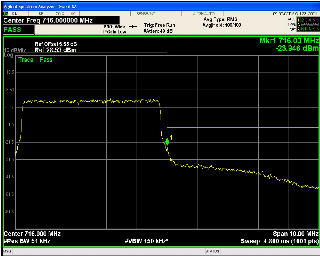
Band17 QPSK BW=10MHz Channel=23780 RB Size=50 Position=#0
