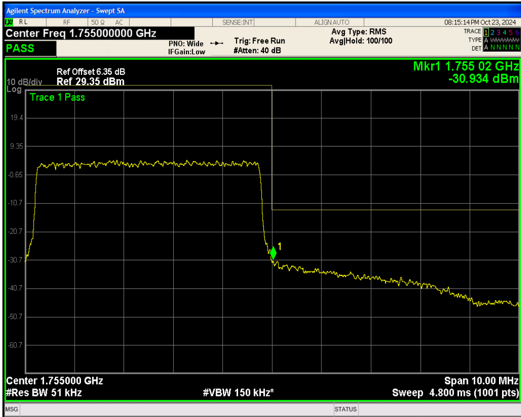
Band4 16QAM BW=5MHz Channel=20375 RB Size=25 Position=#0
