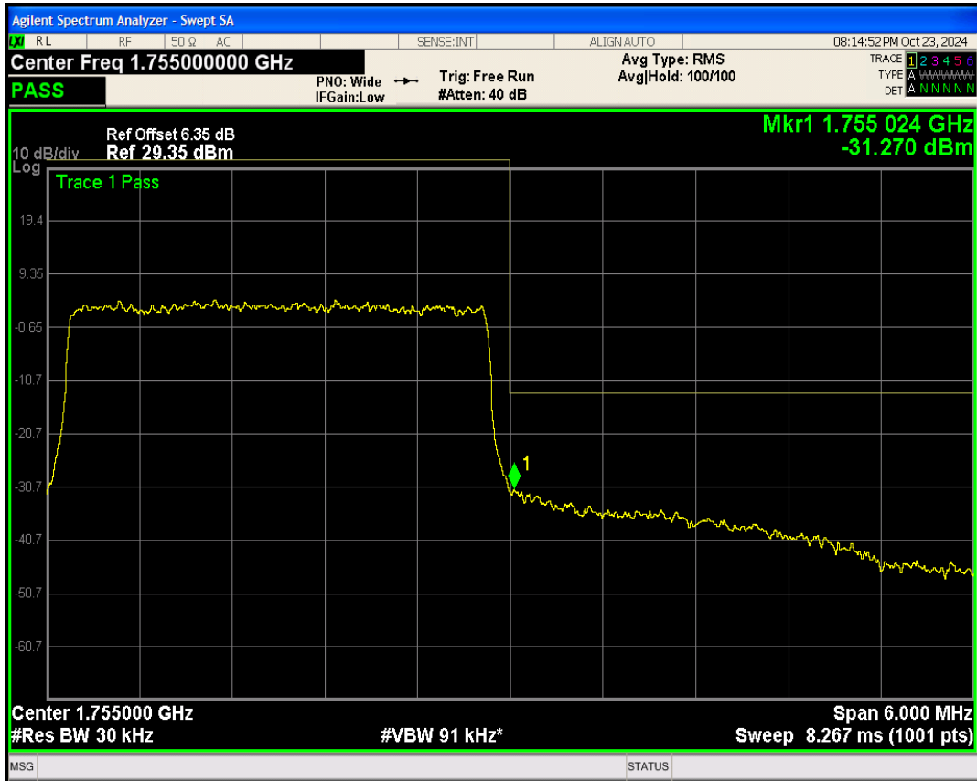
Band4 16QAM BW=3MHz Channel=20385 RB Size=15 Position=#0
