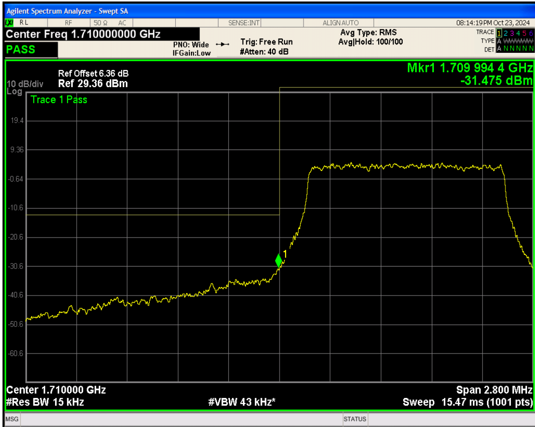
Band4 16QAM BW=1.4MHz Channel=19957 RB Size=6 Position=#0
