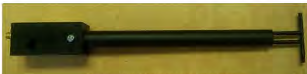
Figure 1 – MVG COMOSAR Validation Dipole
