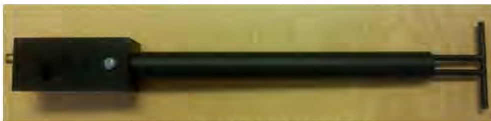
Figure 1 – MVG COMOSAR Validation Dipole
