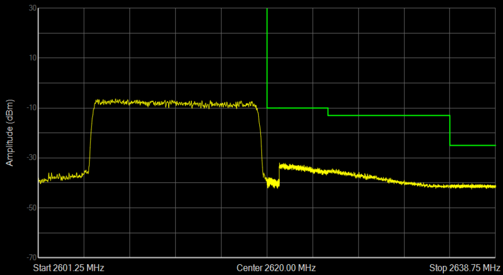
Band38 QPSK BW=15MHz Channel=38175 RB Size=75 Position=#0
