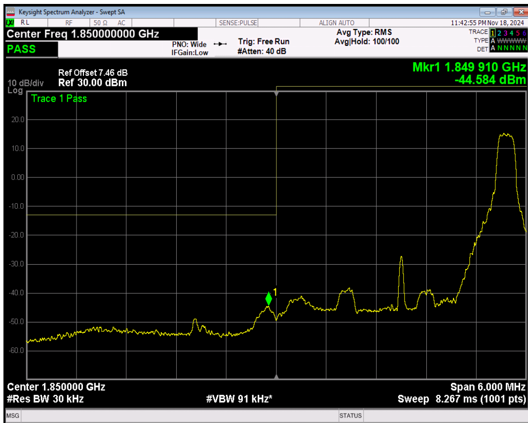
Band25 16QAM BW=3MHz Channel=26055 RB Size=15 Position=#0
