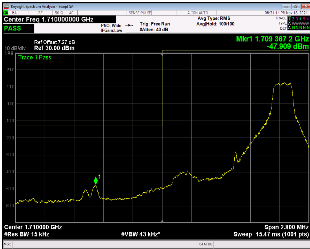
Band4 QPSK BW=1.4MHz Channel=19957 RB Size=6 Position=#0
