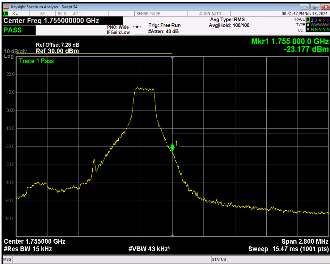
Band4 QPSK BW=3MHz Channel=19965 RB Size=1 Position=#0
