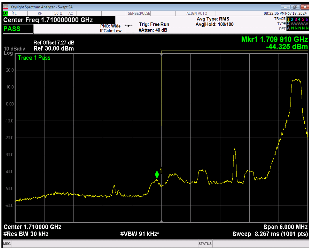
Band4 16QAM BW=3MHz Channel=19965 RB Size=15 Position=#0
