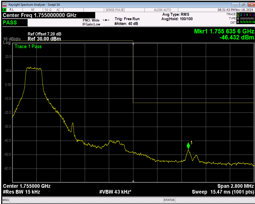
Band4 16QAM BW=1.4MHz Channel=20393 RB Size=1 Position=#Max
