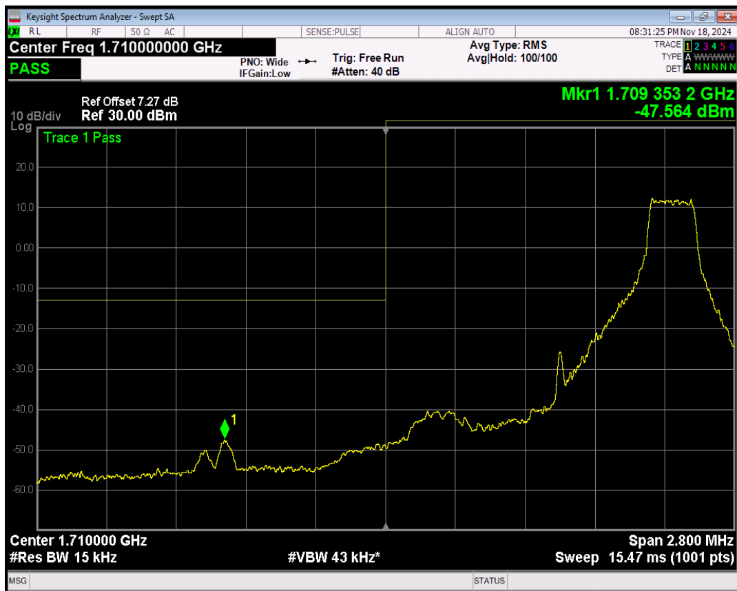
Band4 16QAM BW=1.4MHz Channel=19957 RB Size=6 Position=#0
