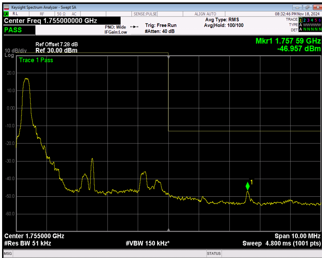
Band4 QPSK BW=5MHz Channel=20375 RB Size=1 Position=#Max
