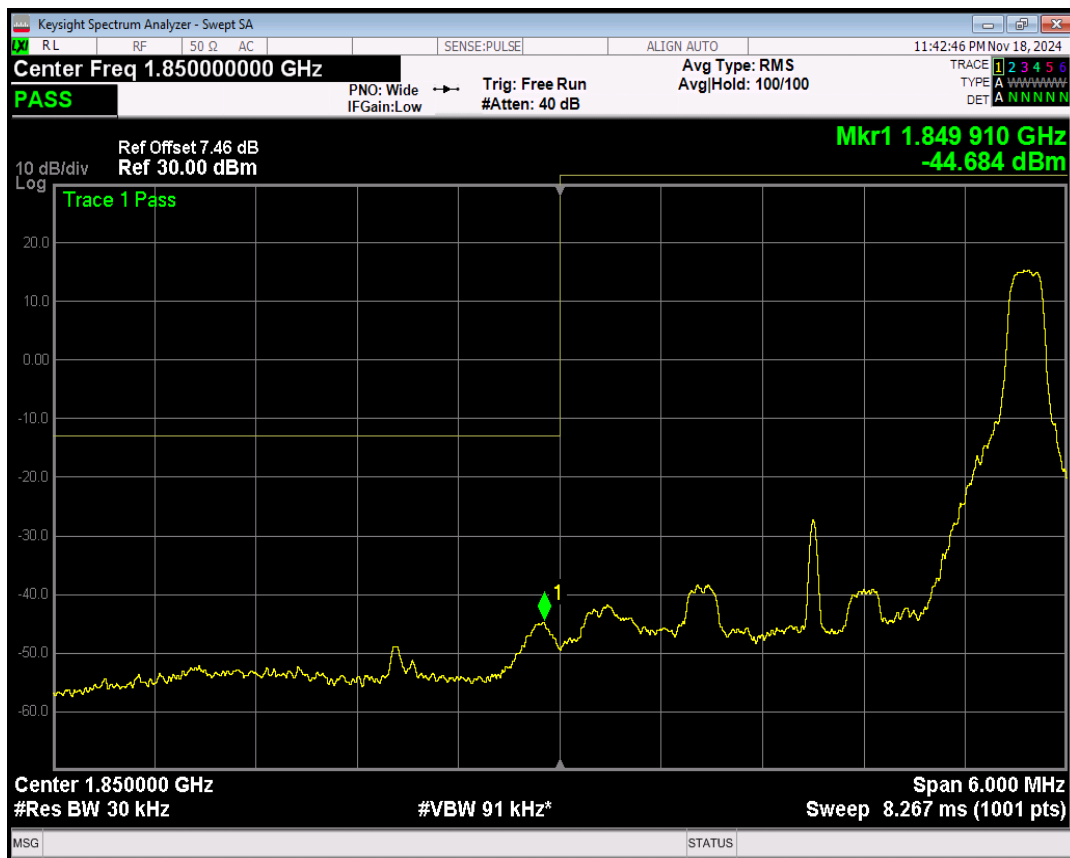
Band25 QPSK BW=3MHz Channel=26055 RB Size=1 Position=#0
