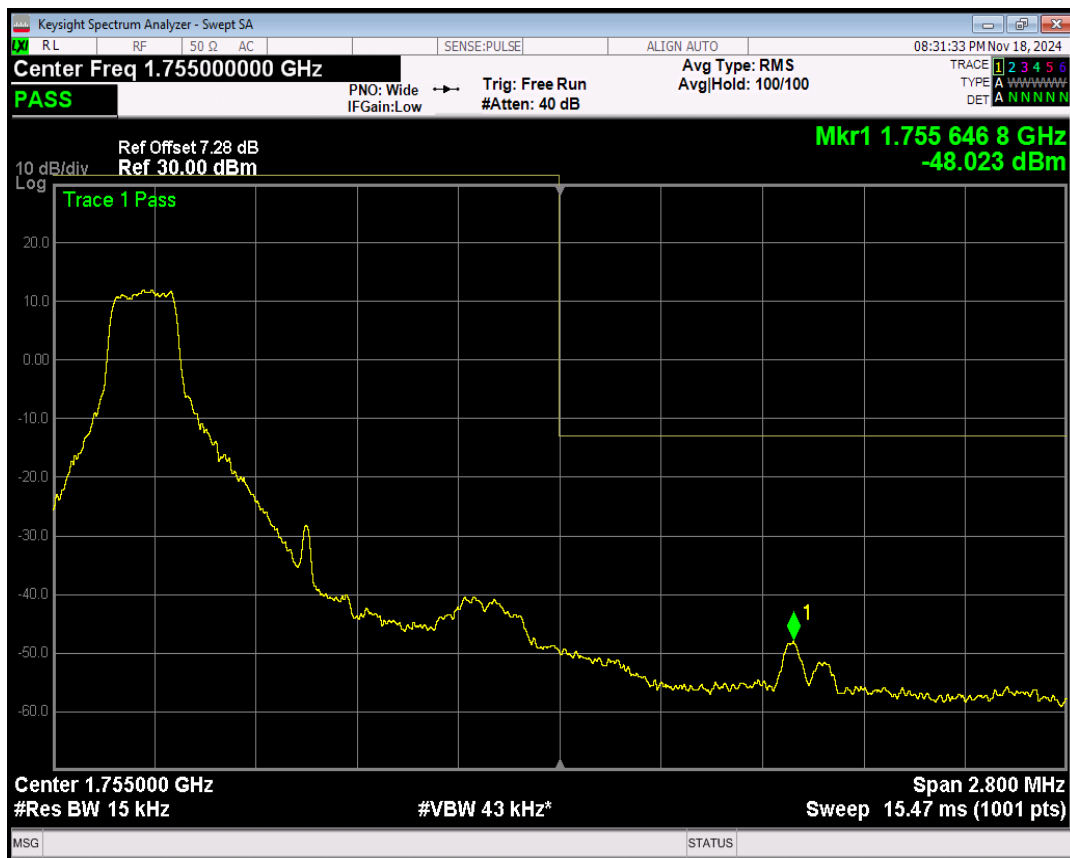
Band4 QPSK BW=1.4MHz Channel=20393 RB Size=1 Position=#Max
