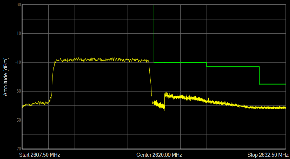
Band38 QPSK BW=10MHz Channel=38200 RB Size=50 Position=#0
