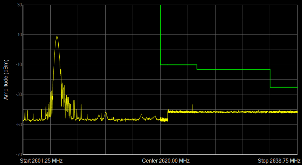
Band38 QPSK BW=15MHz Channel=38175 RB Size=1 Position=#0
