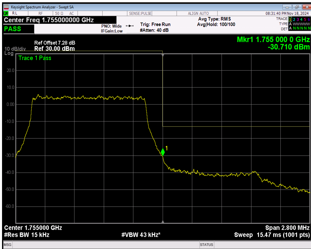
Band4 16QAM BW=1.4MHz Channel=20393 RB Size=1 Position=#0
