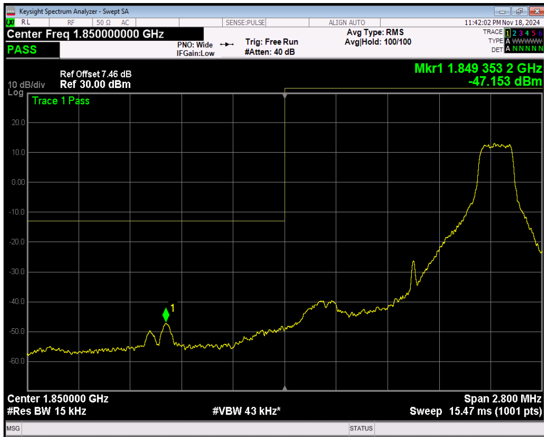
Band25 QPSK BW=1.4MHz Channel=26047 RB Size=6 Position=#0
