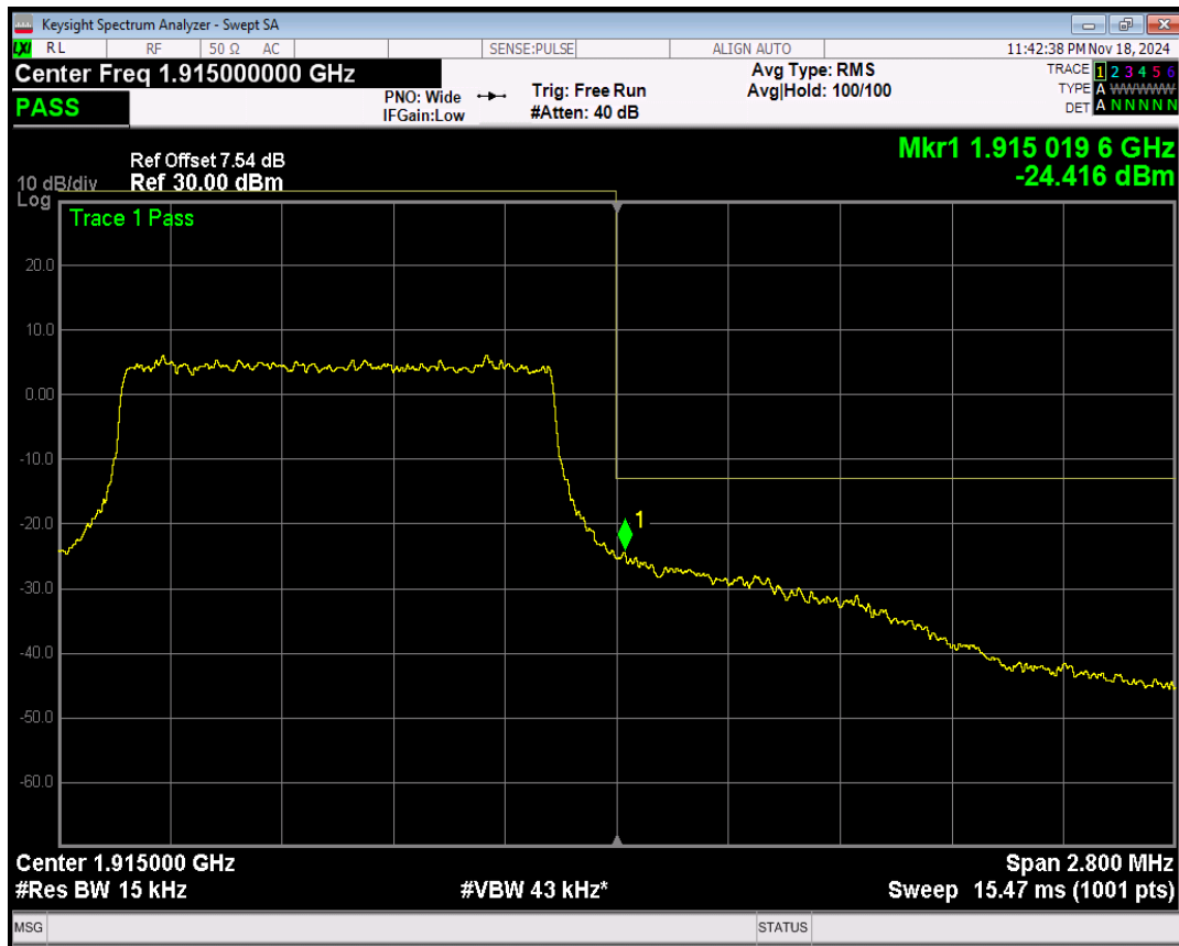
Band25 QPSK BW=3MHz Channel=26055 RB Size=1 Position=#Max
