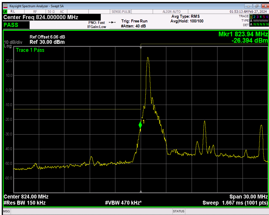
Band26(824-849) QPSK BW=15MHz Channel=26865 RB Size=75 Position=#0
