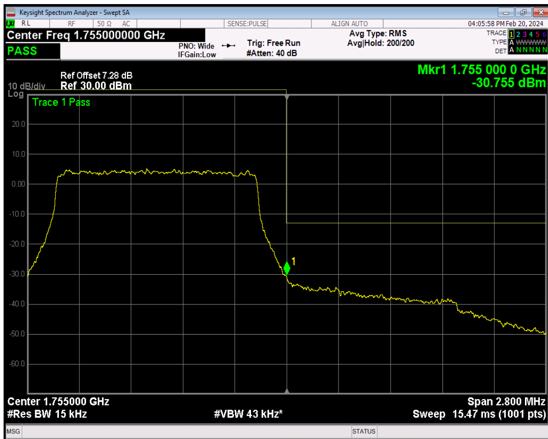
Band4 16QAM BW=1.4MHz Channel=20393 RB Size=1 Position=#0
