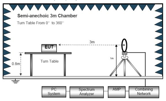
(B) Radiated Emission Test-Up Frequency 30MHz~1GHz
